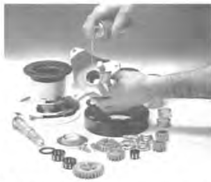
7 (a) Spray inside drum, base and pedestal with CRC6-66 or WD40 and replace bearing race(s) making sure they are properly seated. (b) Lightly grease gears — teeth and bores, clutches, drive shaft, thrust washers and needle roller bearings
