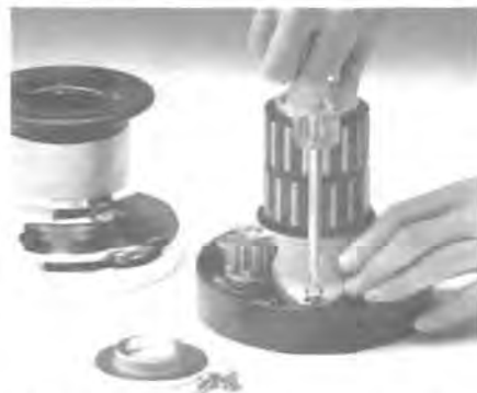
3 Undo cheese head screws — 3 off on models 20 through 27, 4 off on models 28 and 29.
