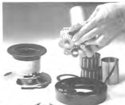
8 (a) Re-assemble parts into pedestal with clutch marked "C" on central shaft for clockwise rotation. For anti-clockwise rotation, assemble clutch marked "A" on to central shaft.
