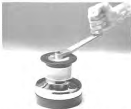
(b) Lightly grease thread and underside of retaining cap, refit and tighten firmly.
