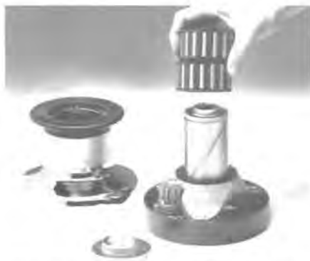
(b) Hold gearing on pedestal, turn pedestal over and align output gear with base and lower pedestal into place. (c) Replace screws and tighten down firmly. 9 (a) Fit thrust washer, main bearing(s) and drum
