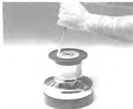
1 Remove retaining cap — tap undone in anti-clockwise direction
