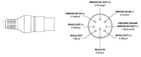
Line up the arrow on the GPS connector with the arrow on the GPS cable and plug together. The pin details are shown for information.
