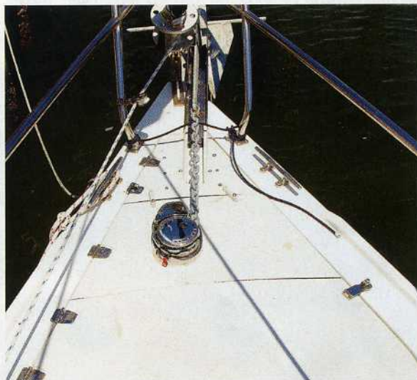
By cutting the anchor-locker lid into sections, Clarence was able to install the windlass and still have access to the locker, at left. Note that he backs up the windlass lock with a safety line through the chain. The anchor locker exposed, at right, shows the wiring and the mounting hinges for the windlass pad installed on both sides.
