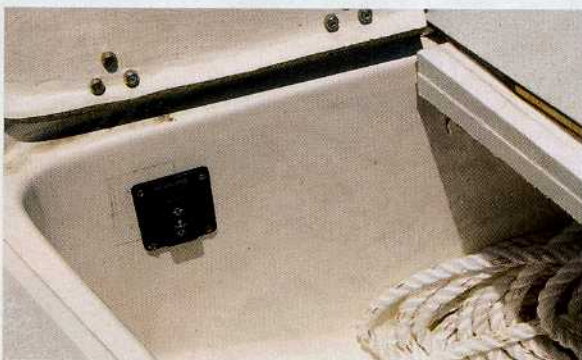
Clarence put the windlass master switch in the anchor locker, above. Note the hatch latches, at right.
