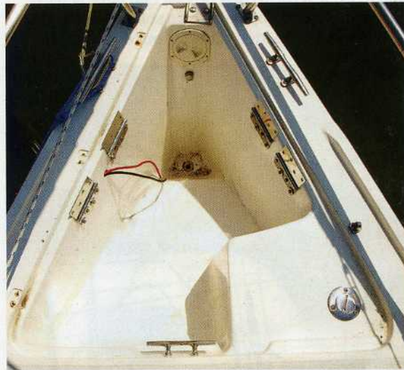
By cutting the anchor-locker lid into sections, Clarence was able to install the windlass and still have access to the locker, at left. Note that he backs up the windlass lock with a safety line through the chain. The anchor locker exposed, at right, shows the wiring and the mounting hinges for the windlass pad installed on both sides.
