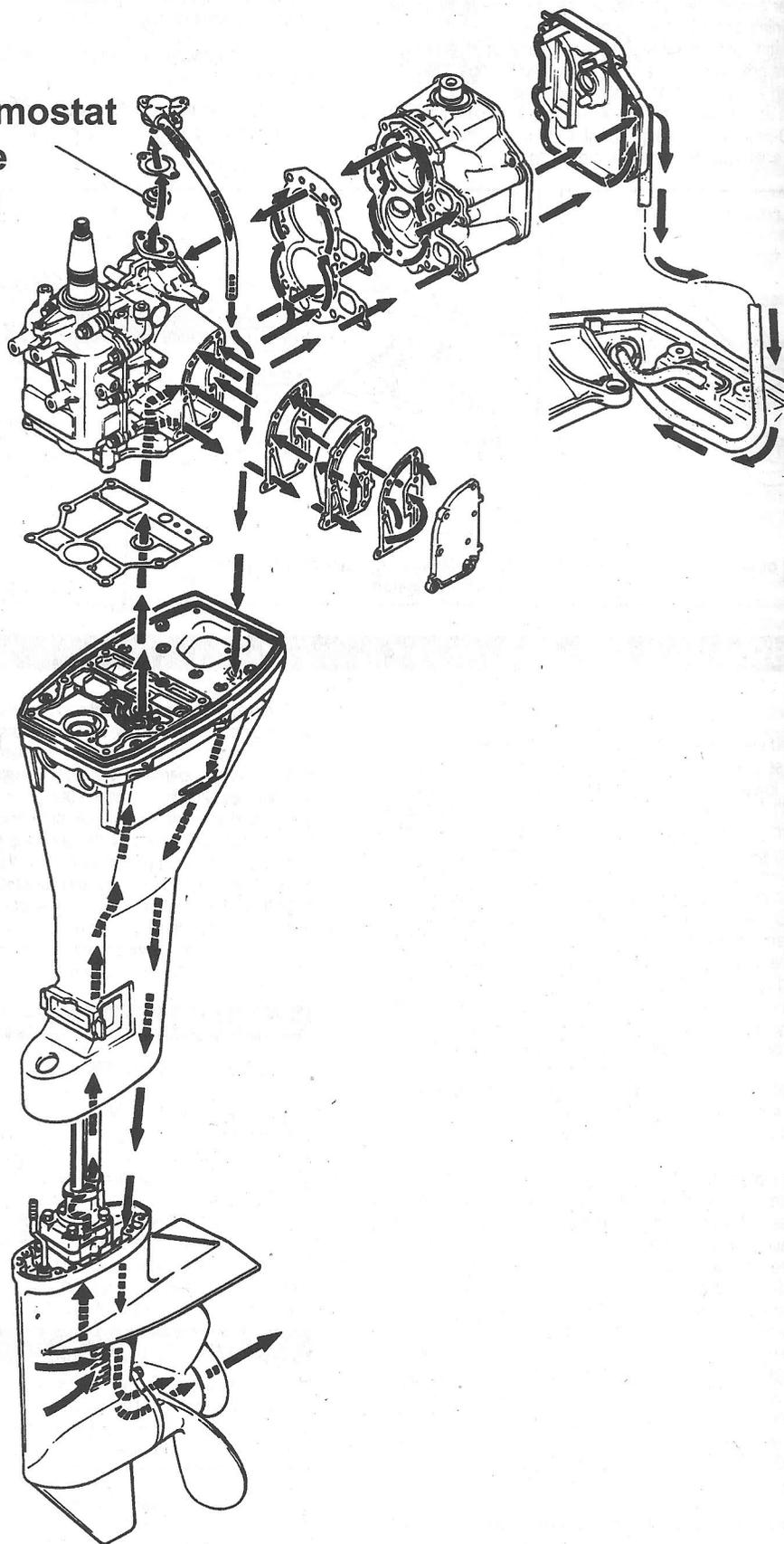
Fig. 174 Cut-away view of a typical outboard cooling system showing water flow - 9.9 hp 4-stroke shown, most other Yamahas similar
