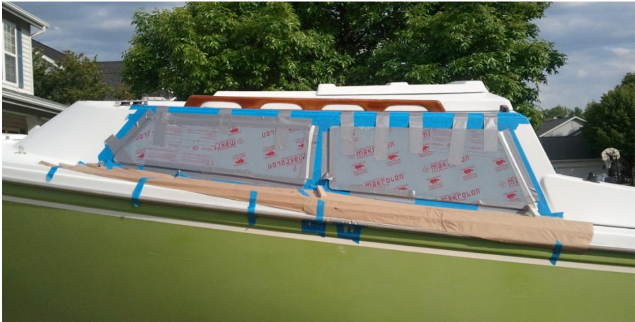
After letting the adhesive cure for three days, I removed the tape and protective covering over the Plexiglas.
