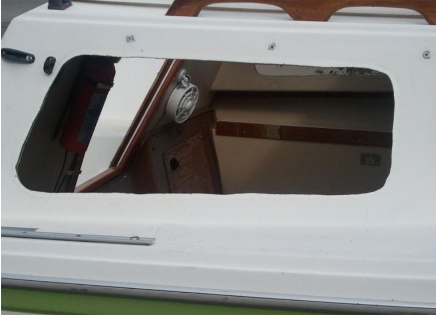
Before I did any cutting on the Plexiglas sheets, I wanted to make sure the drawing of the windows was exactly the right size. I printed the new windows and transferred the images to some poster board that I had lying around. Next I cut the shapes out and placed them over the window openings. They fit exactly like I was hoping they would.
