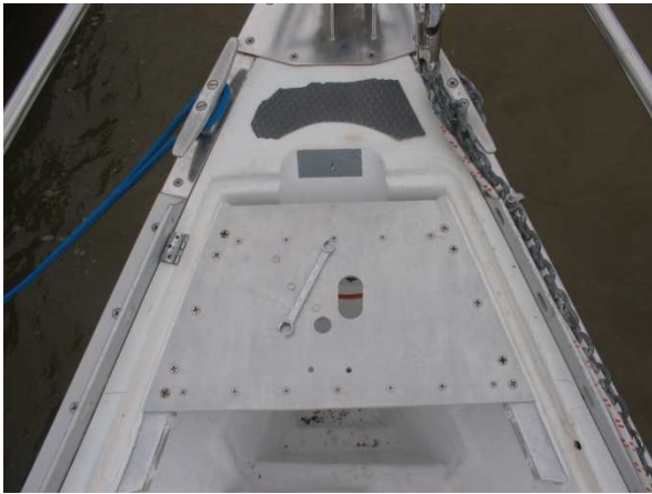
Aluminum plate installed
