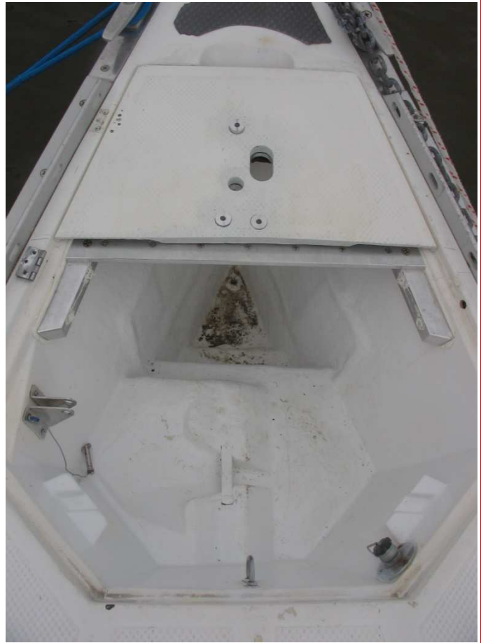
Holes for Lewmar bolts, chain and wiring were drilled using Lewmar paper pattern.
