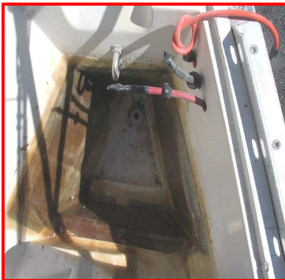
I drilled 3 holes for power cables. Control wire is the one with knot. Grummetts were installed to prevent cutting cables on FB.
