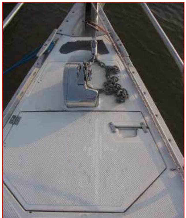
Holes for Lewmar bolts, chain and wiring were drilled using Lewmar paper pattern.
