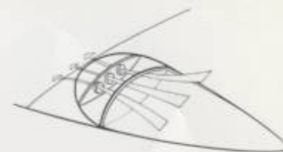
Air intakes streamlined into the roof.
