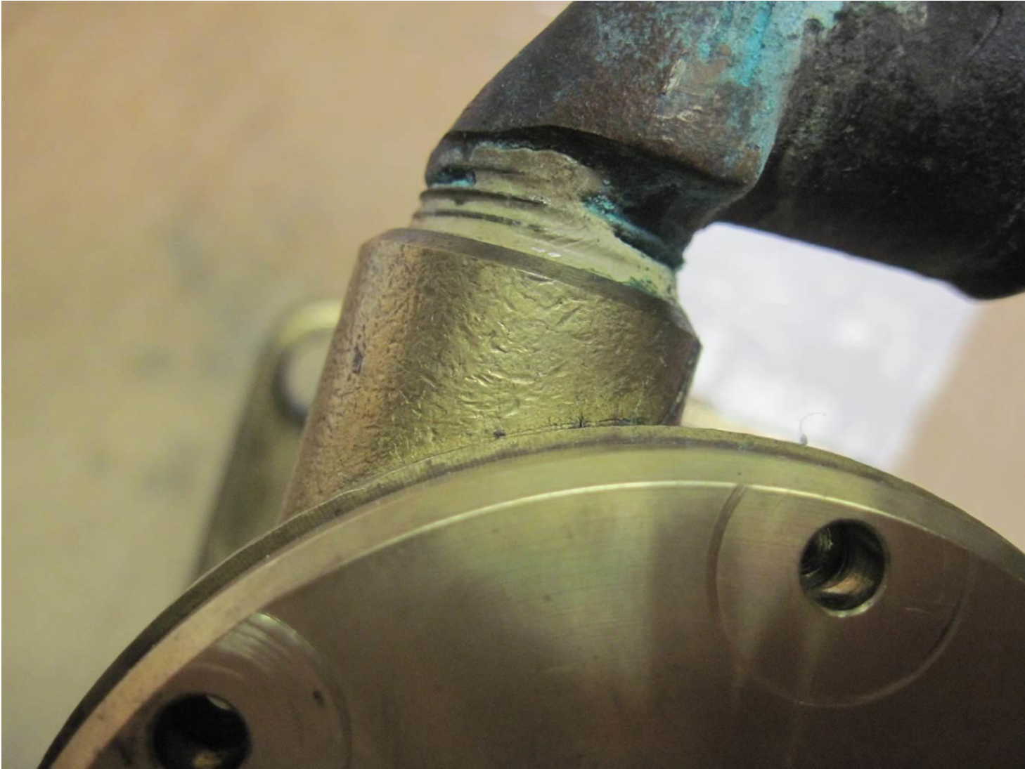
This picture shows the spacing of the cover edge to the pump body edge at the hole side of the plate.
