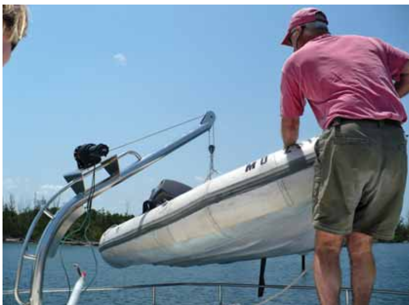
This RIB is lifted by davit onto an aft roof deck that has short rails around the roof ledge, offering those who have height issues something to grab on to.
