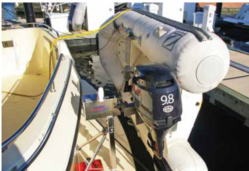
Swim Platform hinge with a rotating outboard bracket keeps the motor upright.
