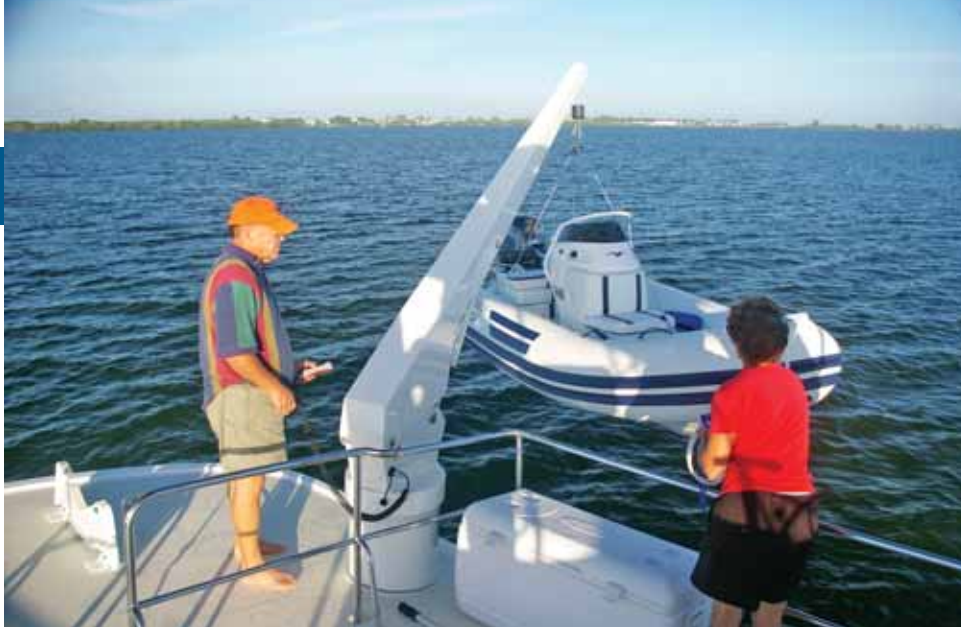
A six-position electro-hydraulic dinghy boom makes launch and recovery very simple.
