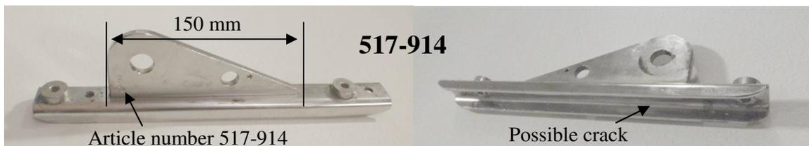
All the failed fittings origin from long distance cruising boats with inadequate rig tune and long periods of sailing using only the genoa.
