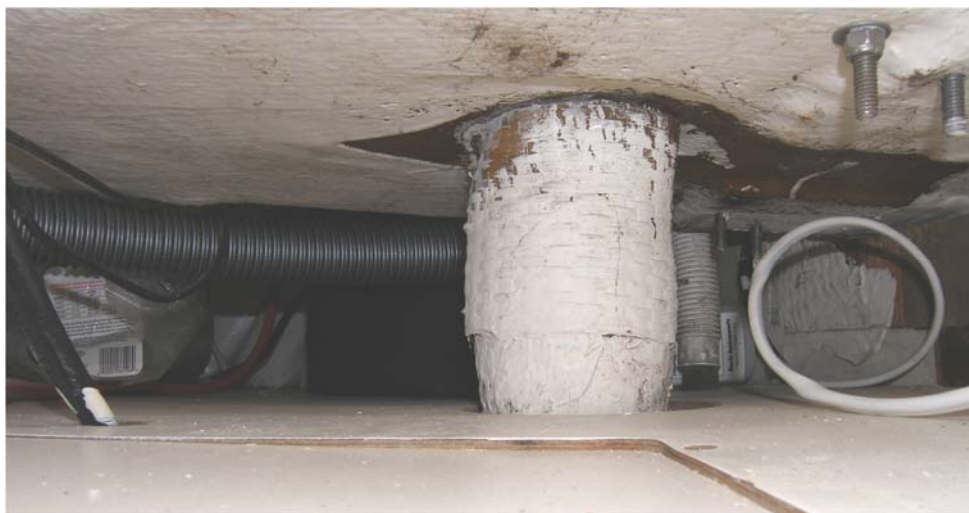
Illustration of “best estimate” of the rudder bearing mounting system.
