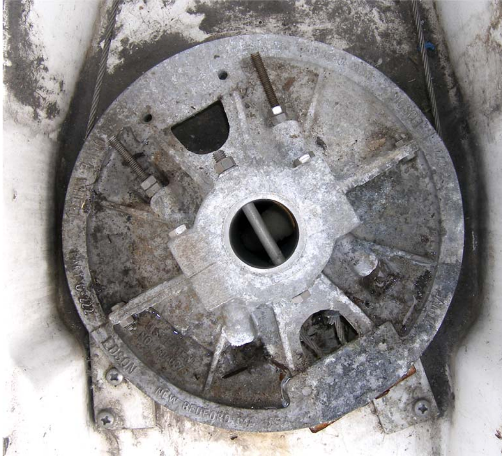
6.5-in (radius) Edson Radial Drive Wheel with deck cover removed.
