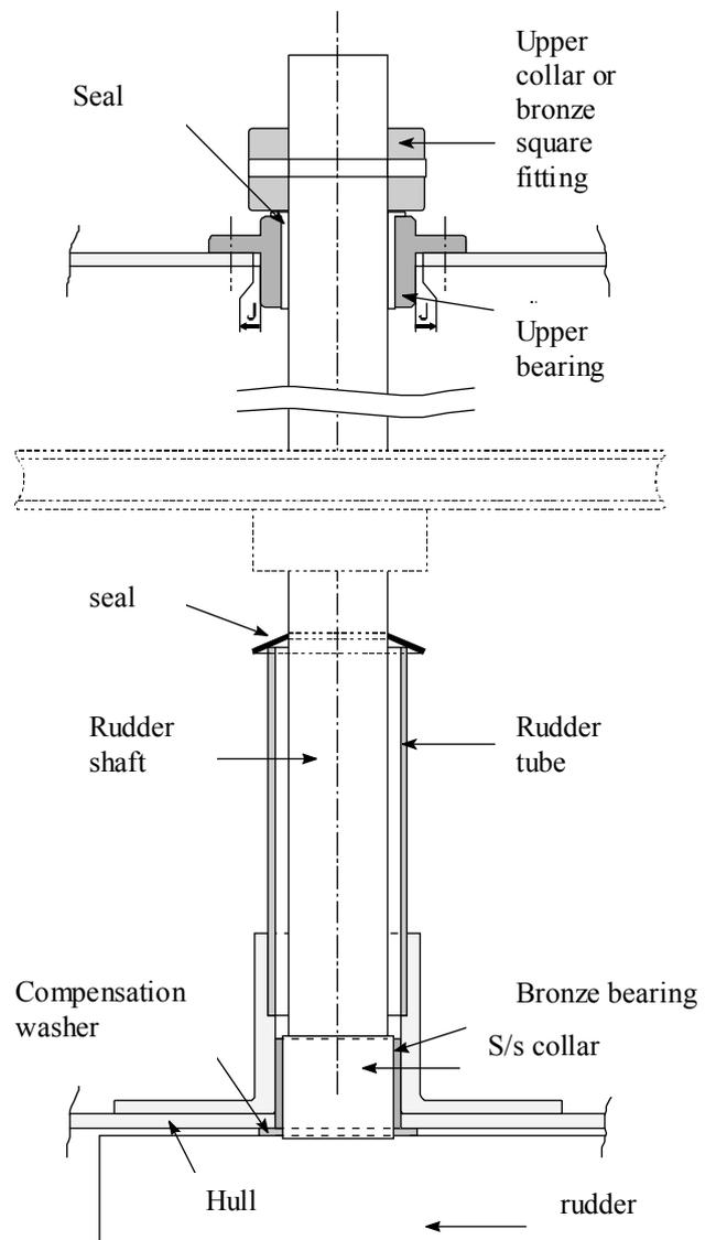
**③ SAILING BOAT SUSPENDED RUDDER ASSEMBLY WITH AUTOMATIC BEARING ALIGNMENT**
