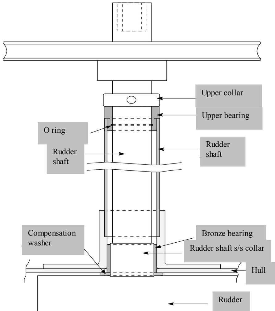
**② SAILING BOAT SUSPENDED RUDDER ASSEMBLY WITH DECK BEARING**
