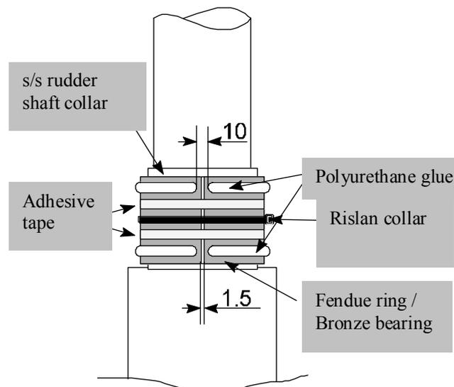
**① SAILING BOAT SUSPENDED RUDDER ASSEMBLY WITHOUT DECK BEARING**
