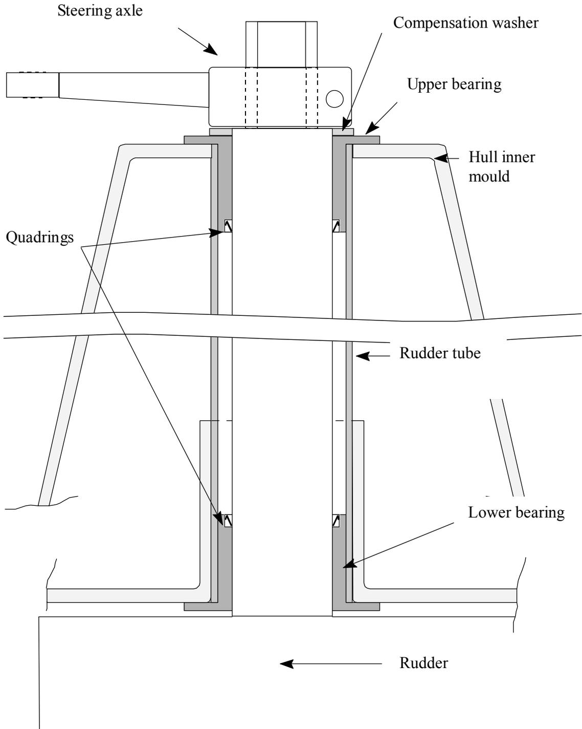
**MOUNTING OF THE RUDDER WITH DECK BEARING FITTED ON THE BRACKET**
