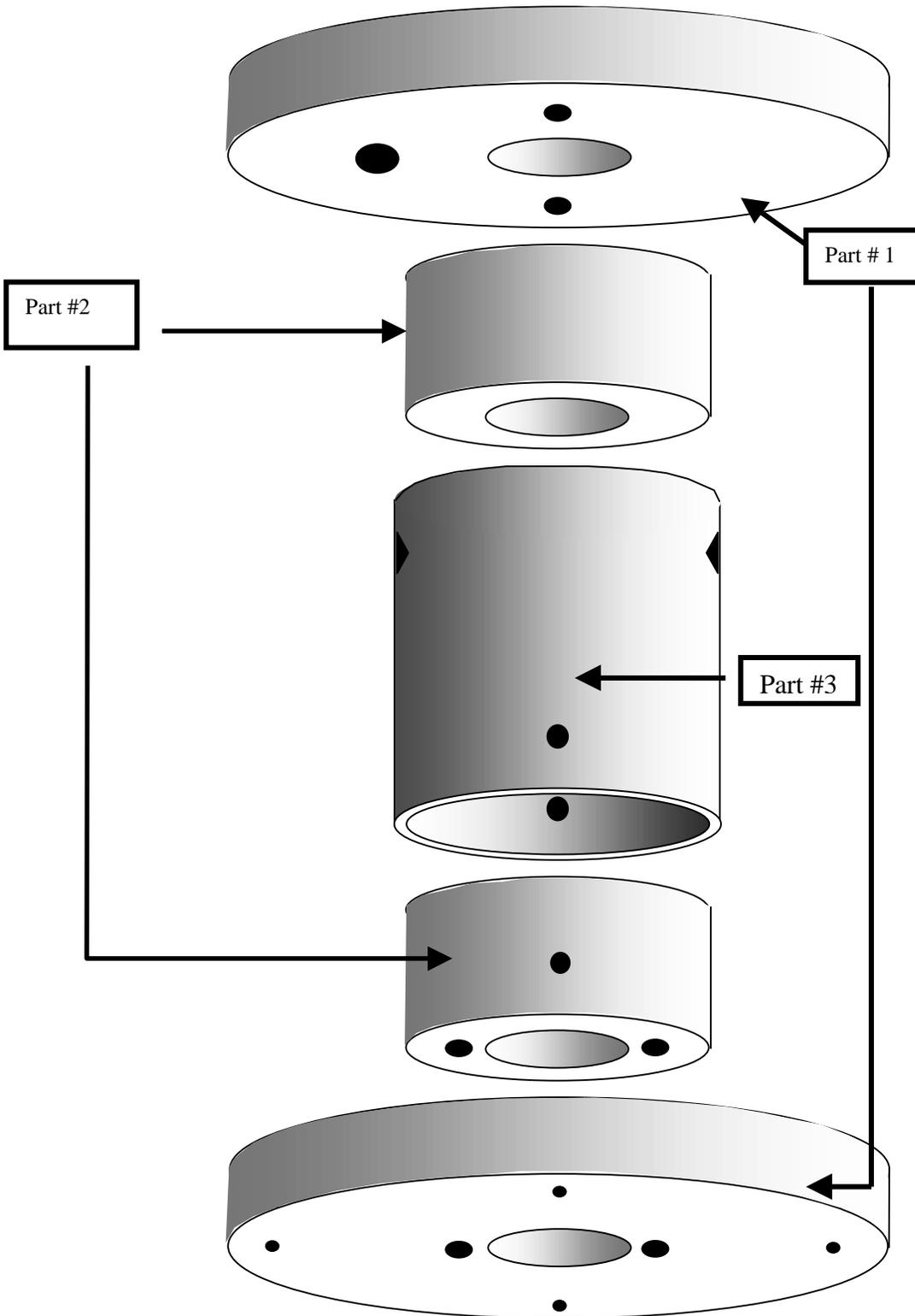
Assembly 2: Parts for base, and pilot holes for screws.
