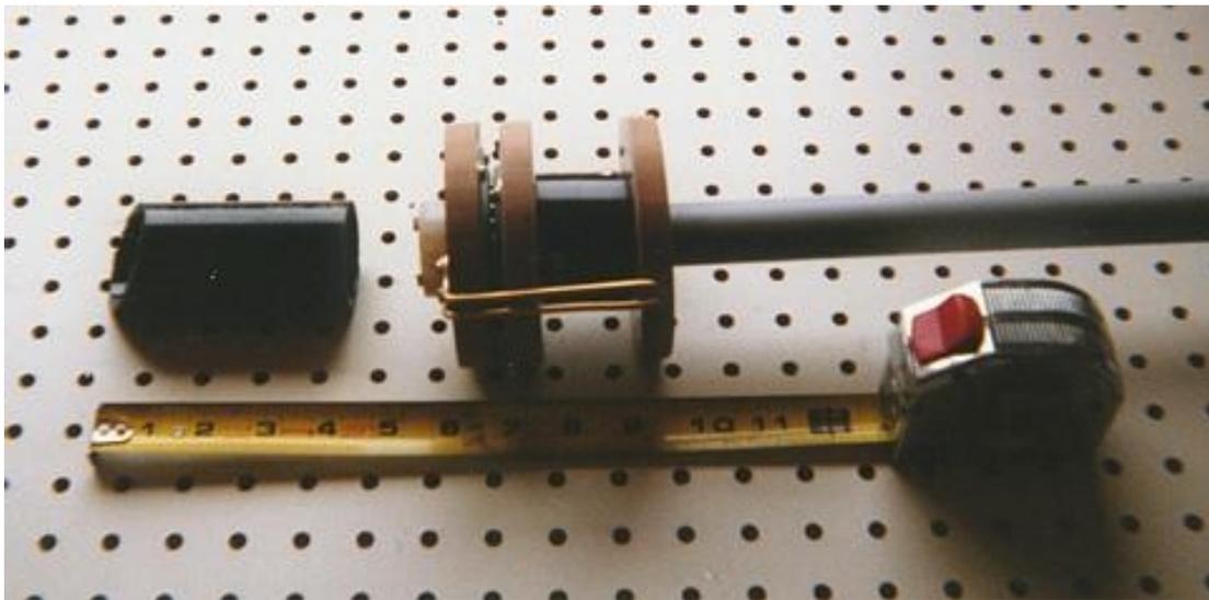
Assembly 1: Parts for drum, and pilot holes for screws.
