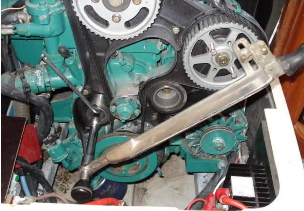
Let's bring the belt to the proper tension now.
