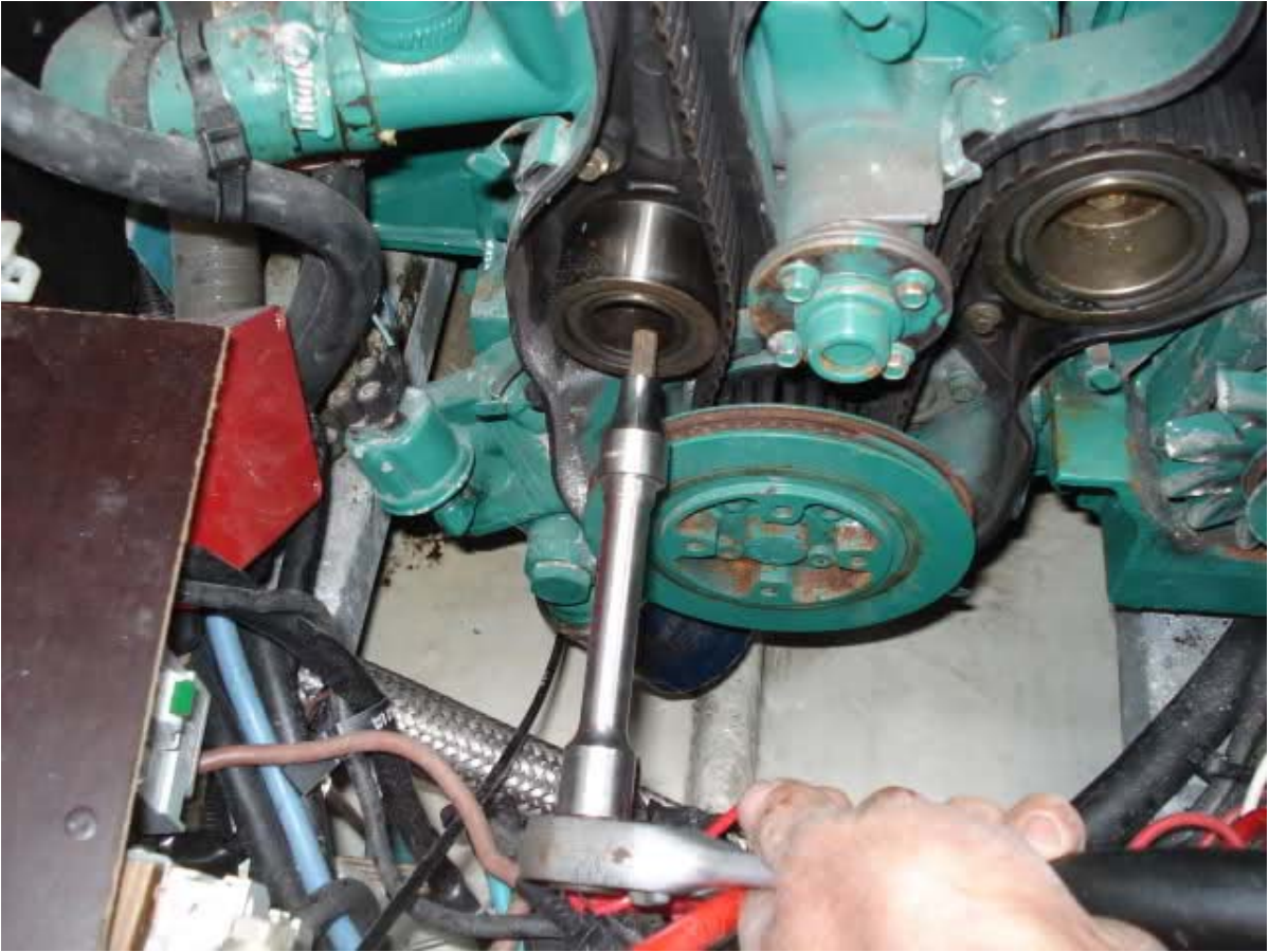
Time to release the tensioner.
