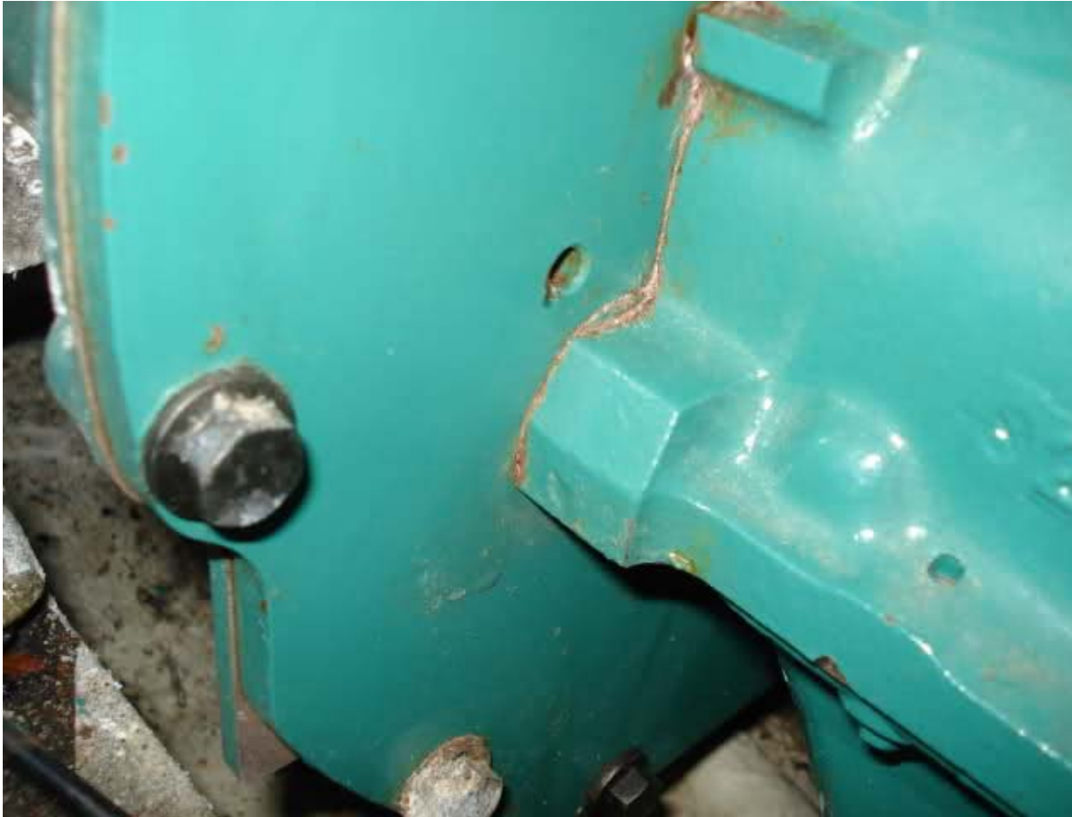
This is the location for the crank/flywheel locking . It's on the back- lefthand side of the engine when you're facing the timebelt. Trial and error will lead you to an agreemeent between cam and crank
