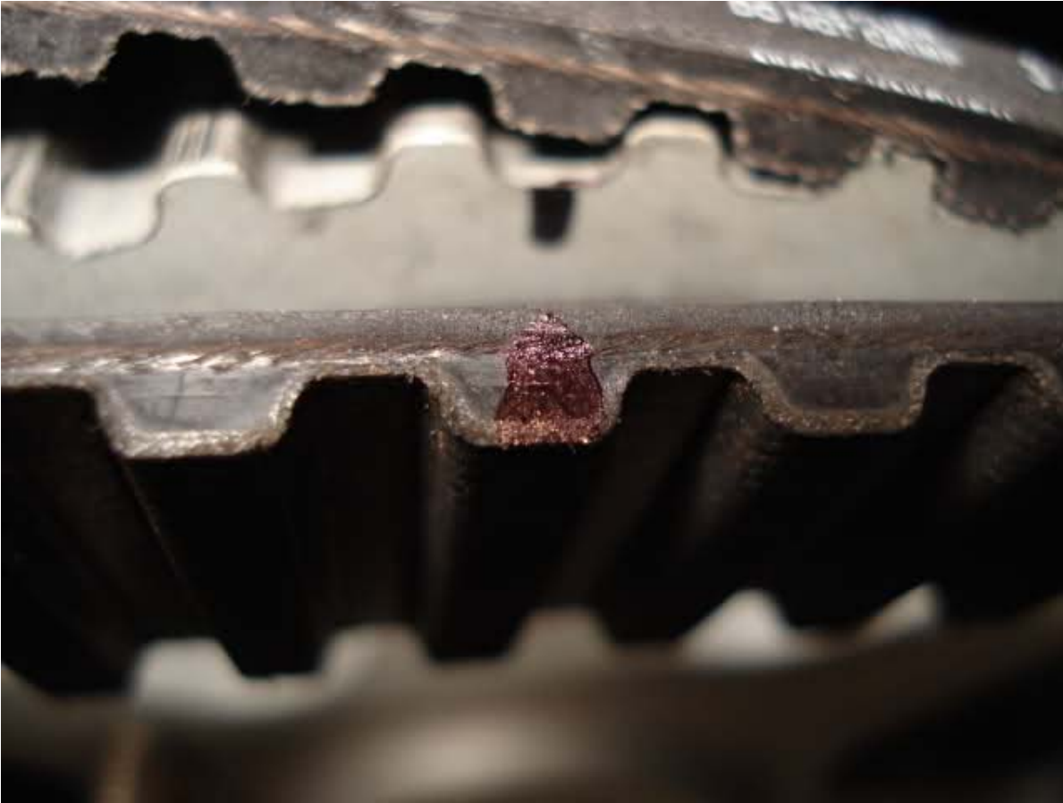
I even put marks on the old belt so I could easily count the number of teeth and compair it with the new installed belt afterwards.
