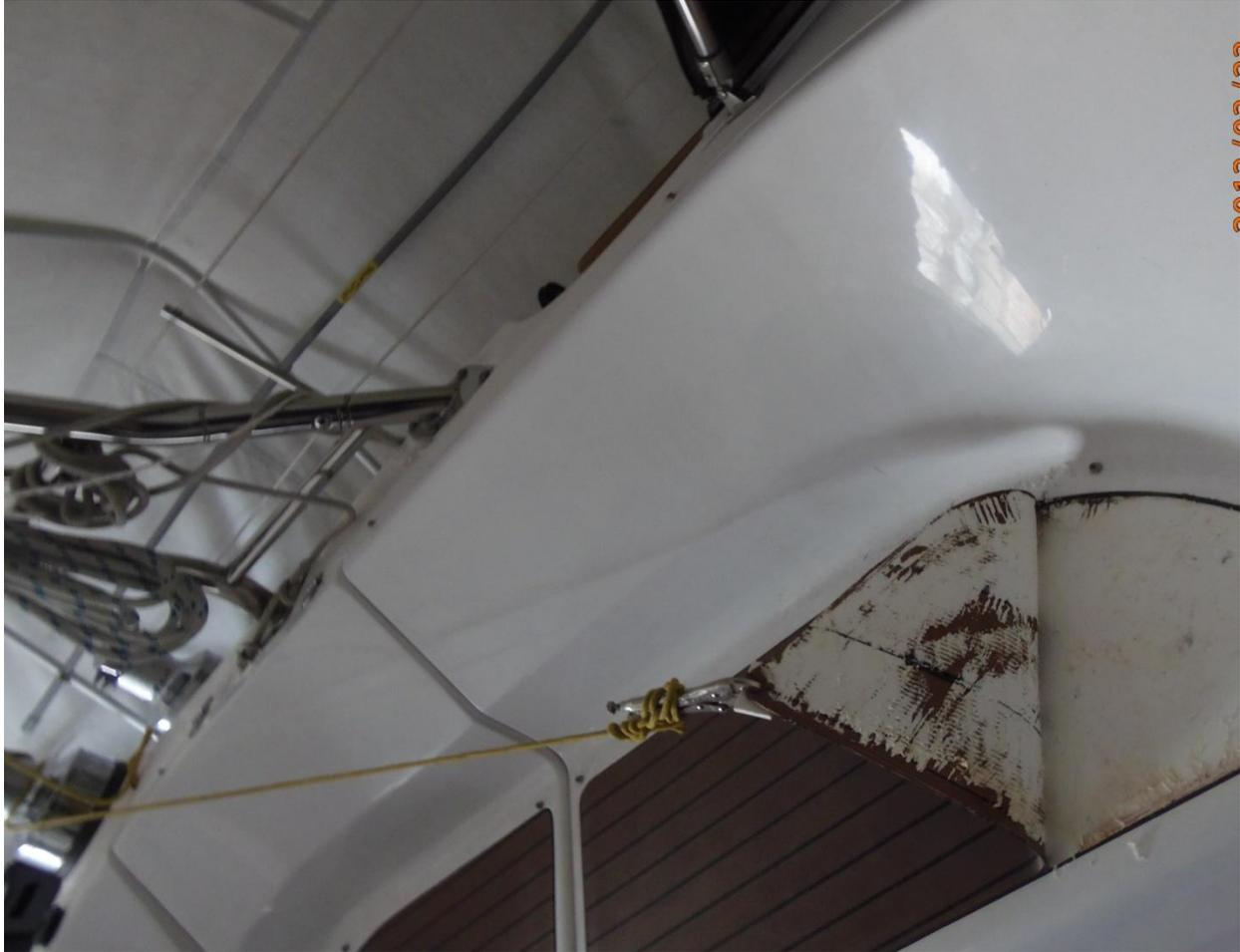
Each pass you make relieves about 1 ½ inches of glue. It takes about 1 minute to make the cut. The reason this works so well is because you are bending the flex teak back almost 180 degrees, which fully exposes the glue line. It literally slices through the 5200 like butter.
