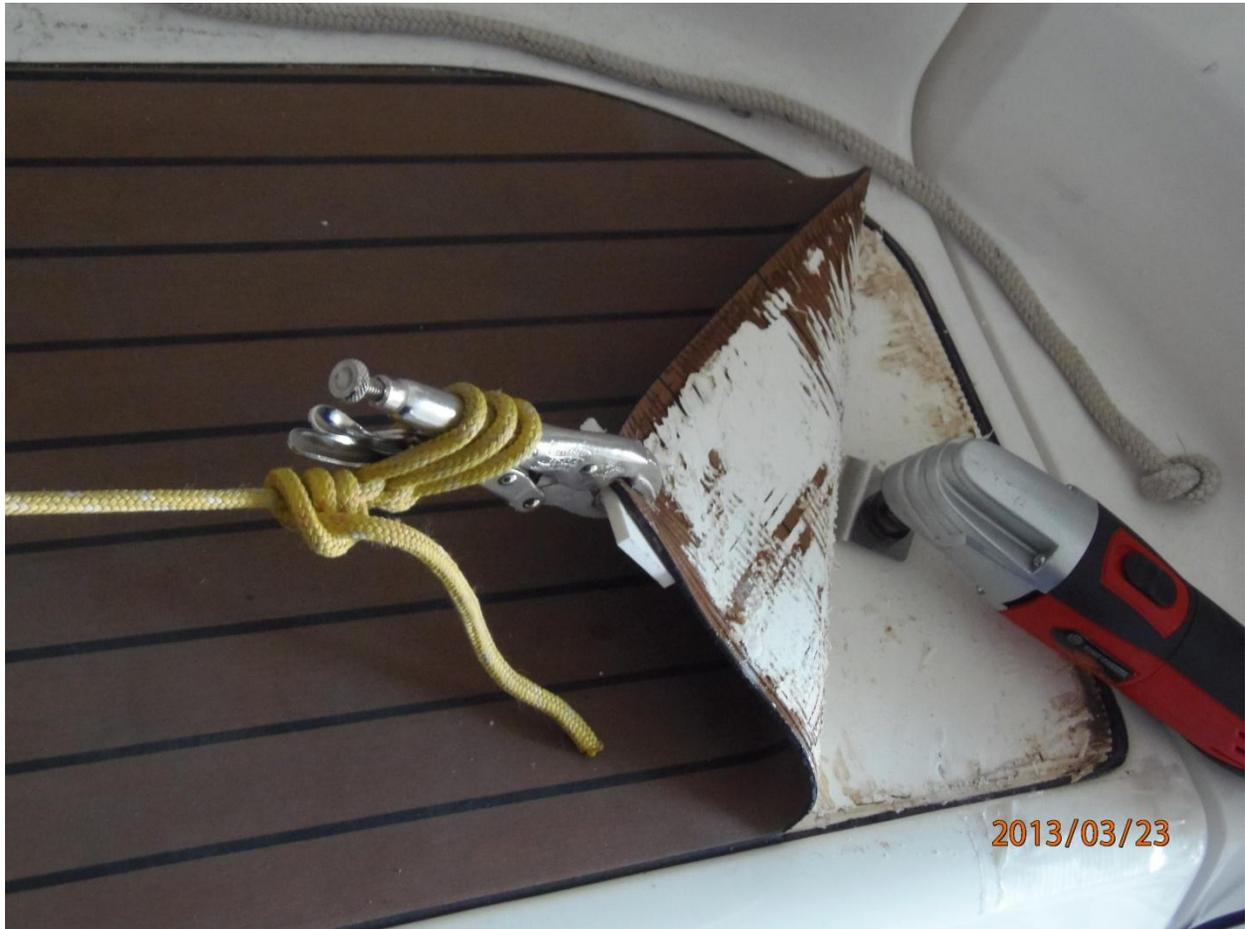
As you do this, the tension in the line will act as a spring, and start to peel back the flex teak as you relieve the exposed glue. You can cut about 1 ½ " of 5200 in one pass.
