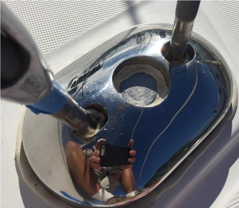
And after filling the center hole on top of the chainplate cover with marine grade silicon. It is the only silicon used in this job. I didn't use butyl since there was no way to secure it. I figure this small amount of silicon won't be too bad to remove the next time I take things apart.
