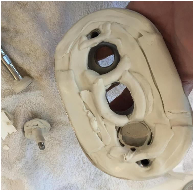
After reinstallation and during the tightening process. Notice the butyl squeezing out:
