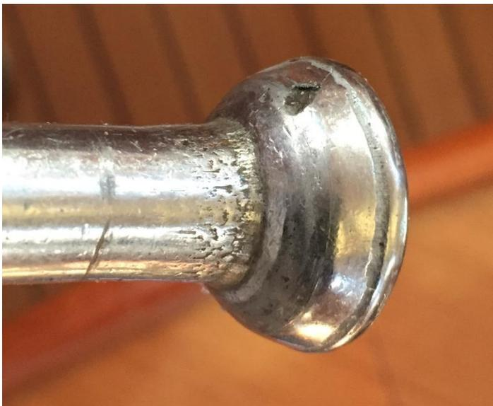
The port tie rod turnbuckle and clevis pin were clearly affected by the water that got in via leakage.
