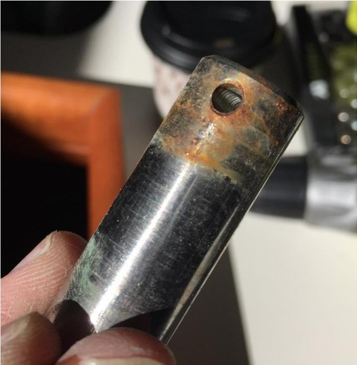
Here is what the starboard side chainplate cover looked like upon removal. There wasn't any meaningful silicone between the deck and the cover. No wonder I had leakage but thankfully no corrosion.
