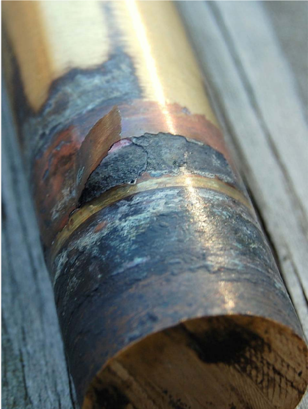
Below is the finished product after installing three new rings of GTU packing.
