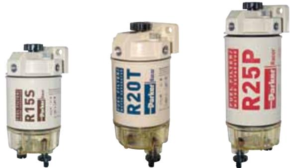
Racor's 200 series fuel filter water separators are specifically designed to handle today's tough diesel filtration problems. These units feature a standard in-head fuel priming pump and are different from one another only in flow capacity and element size.
