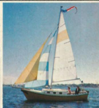
Without sacrificing its traditional character, the 23 incorporates such modern features as a retracting keel, positive foam flotation, a self bailing cockpit, a pop top for full cabin headroom, and the highest quality fiberglass construction. It has berths for five, and is fast, seaworthy and comfortable.
