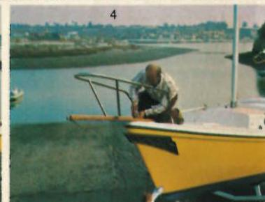
RAISING THE MAST (1) The mast is slid to the rear and the base of the mast is pinned to the hinged mast step. The side shrouds and backstay always remain connected and adjusted for sailing. Only the headstay need be disconnected for trailering. (2) & (3) The
