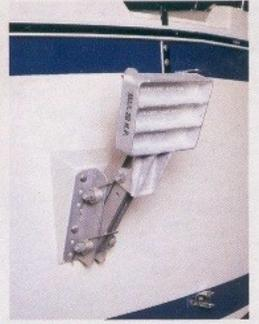
Standard Cruiser specifications include teak toe rails, flush forward hatch, two-tone decks, Bariat winches, and alloy outboard brackets.
