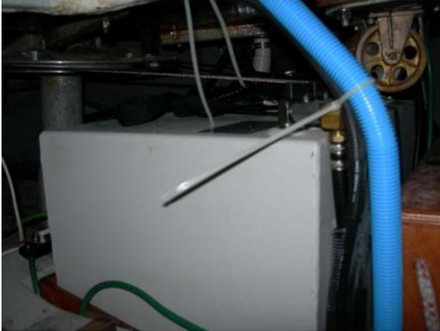
View from Port side showing inspection port and straps over tank that are attached to footman loops on the front of the cradle and a fiberglass boat rib on the back. Inspection port has is well position to pump a fuel sample out to check for water in the tank each spring. You can see cradle at the bottom.
