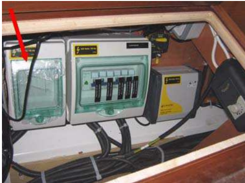
Differential switch 40A - Chart table unit
