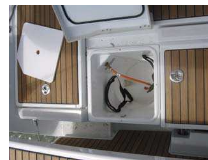
Gas cylinder locker
