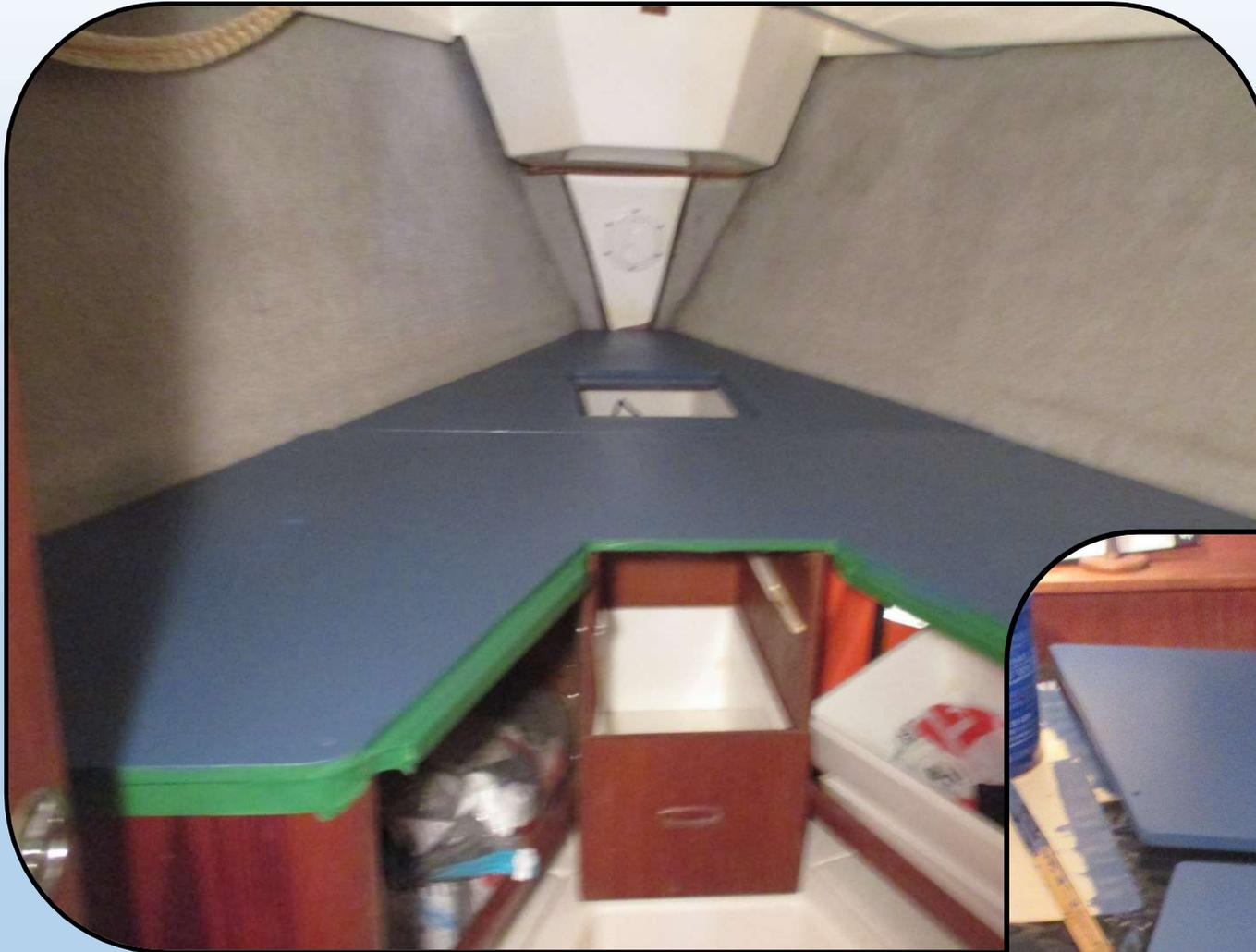
I filled the void above the screw heads & the previous holes for pins with plastic wood, sanded, & then painted the floor bed
