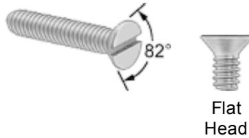
Each screw has an 82° bevel under the head. Sizes noted below have an undercut head to allow more threading. Screws up to 2" long are fully threaded; those longer than 2" have at least 1 1/2" of thread. Length is measured from the top of the head.
