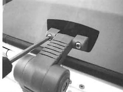
1.3) Undo hinges and release lid from Lower Frame
