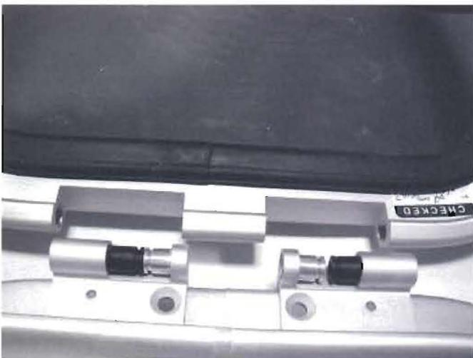
1.5) Remove the screws from one side of each join in the Upper Frame
