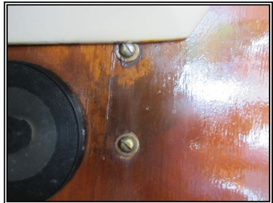
*Additional water damage was found at the base of this bulkhead as viewed from the*
