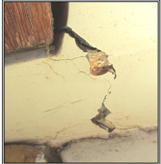
*and cabin sole had focused stresses in this one area. Though these were considered consistent with even minor fore and aft hull flexing, repairs are highly recommended at this time (ER).*
