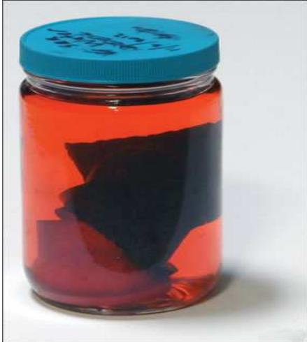
The joker valves were exposed to various chemicals to determine resistance. Exposure time varied, depending on the chemical.
