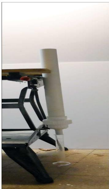
Testers filled a 30-inch stand pipe with water and measured leakage. This setup created back pressure equivalent to the rise from a joker valve to a holding-tank inlet.
