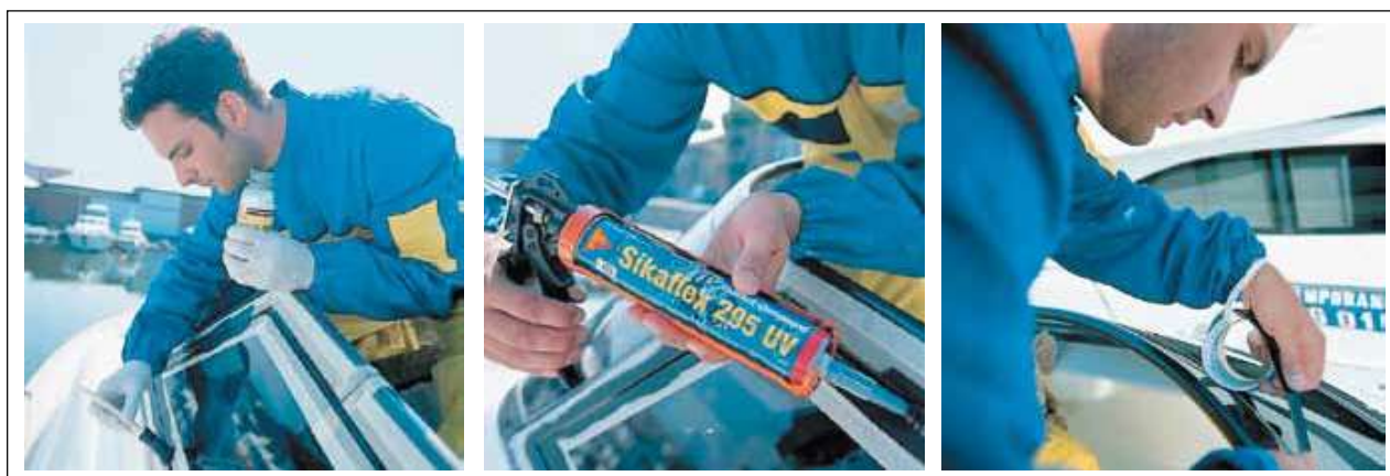
Fig. 123 (a, b & c) Examples of adhesively bonded organic glazing using Sikaflex®-295 UV in conjunction with UV Shielding Tape
