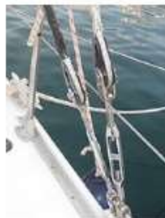
Figure 4: HMPE stranded rope rigging (Dynice DUX) spliced around special thimbles and attached to (turnbuckles) rigging screws. It should be noted that the shroud in the foreground (without black chafe protection) can easily be fully inspected. Picture courtesy of Colligo Marine
