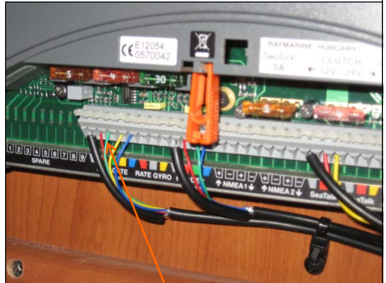
Fluxgate compass wire to course computer
