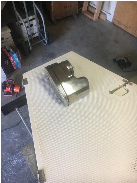
Holes transferred to lid, test fit to locate cut
