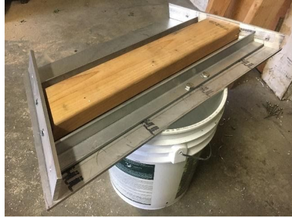
Bolts and jig to hold in place for welding
