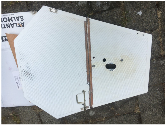
Lid cut in two with nonskid removed at joint
