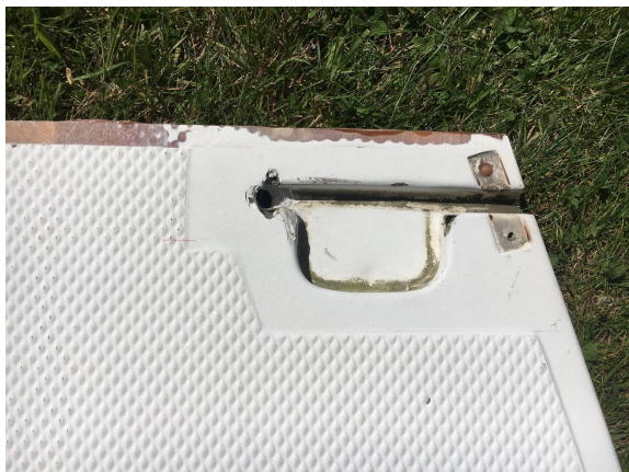
Fiberglass damage at latch
