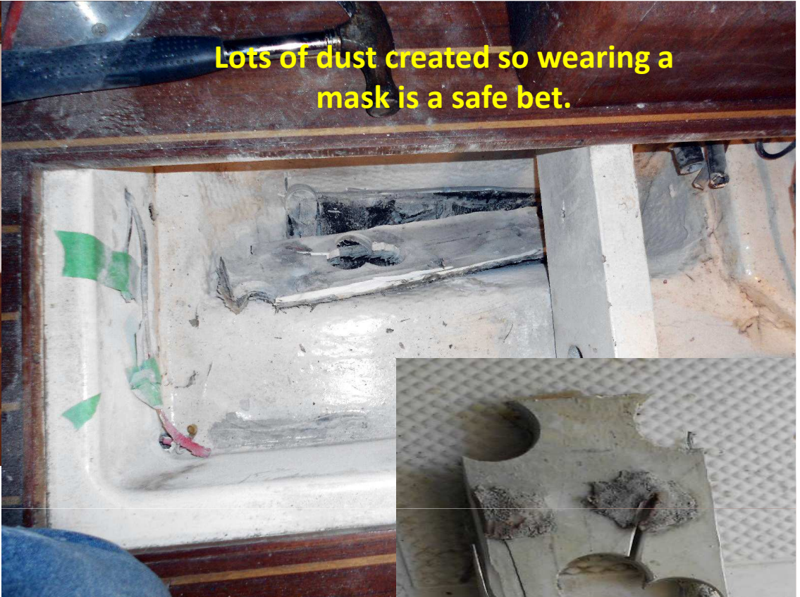
Also using a 4 1/2" cut-off wheel and a multi-tool, I cut alongside the walls.
