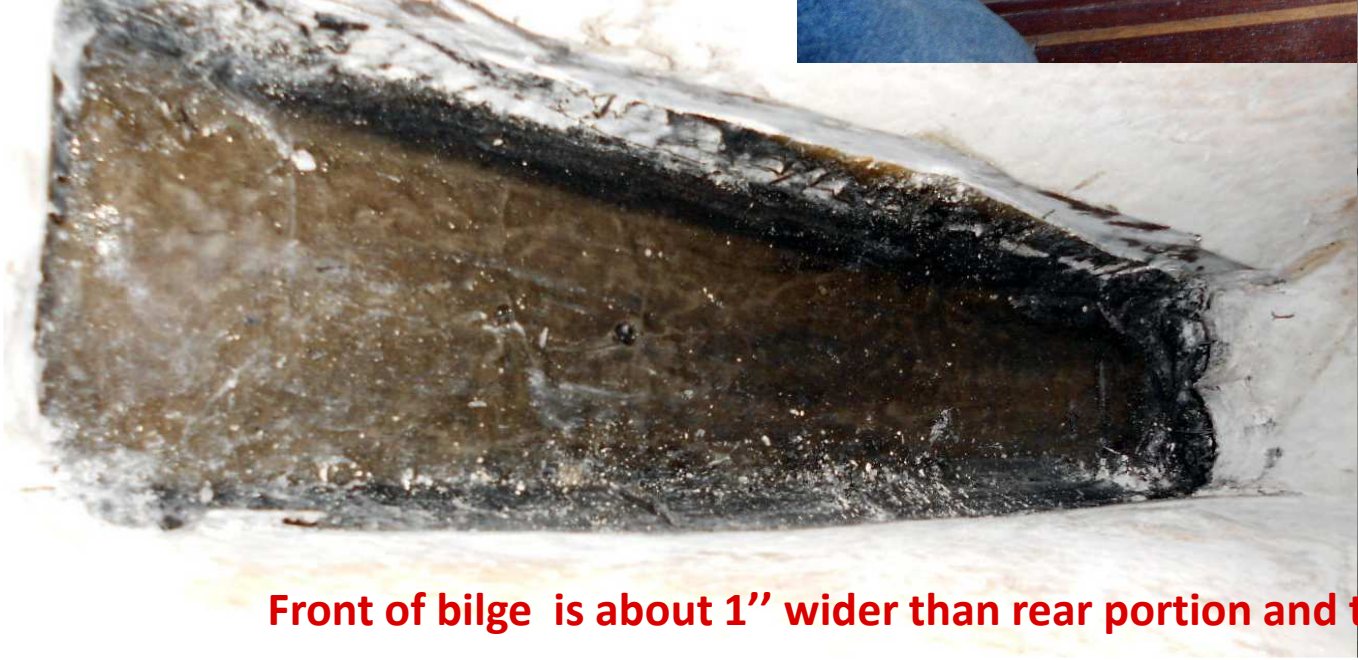
Also using a 4 1/2" cut-off wheel and a multi-tool, I cut alongside the walls.
