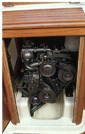
A freshwater cooled Yanmar 27HP diesel provides economical and dependable power.
