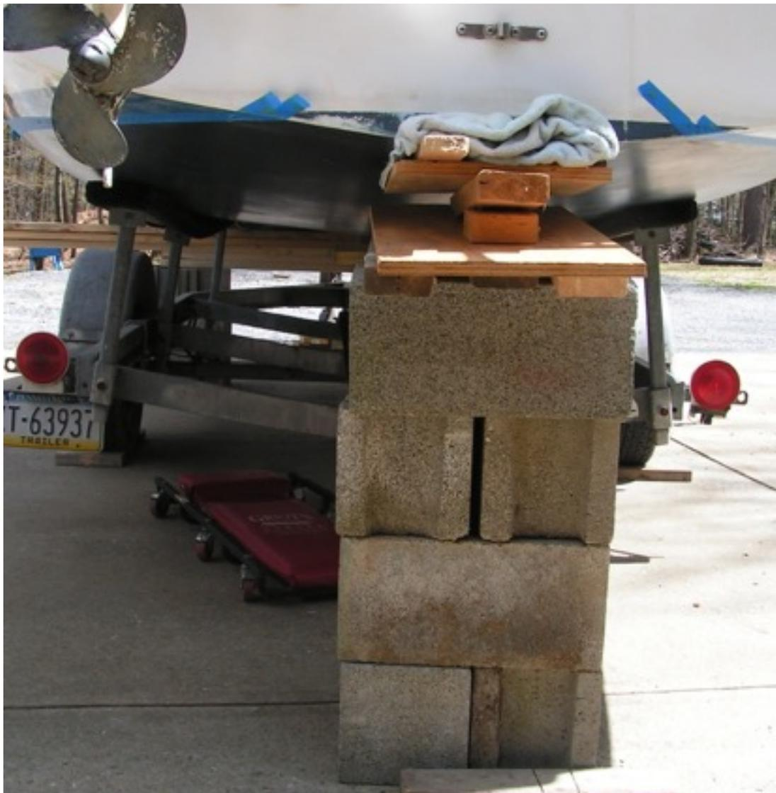
I then started to jack up the tongue of the trailer to raise the bow like I did to the stern but, it seemed to be too much work for the trailer jack so, I used a Ford truck bottle jack further back the trailer from the tongue. Using the auto jack to raise the tongue and using the trailer jack to stabilize the height everything went easy.
