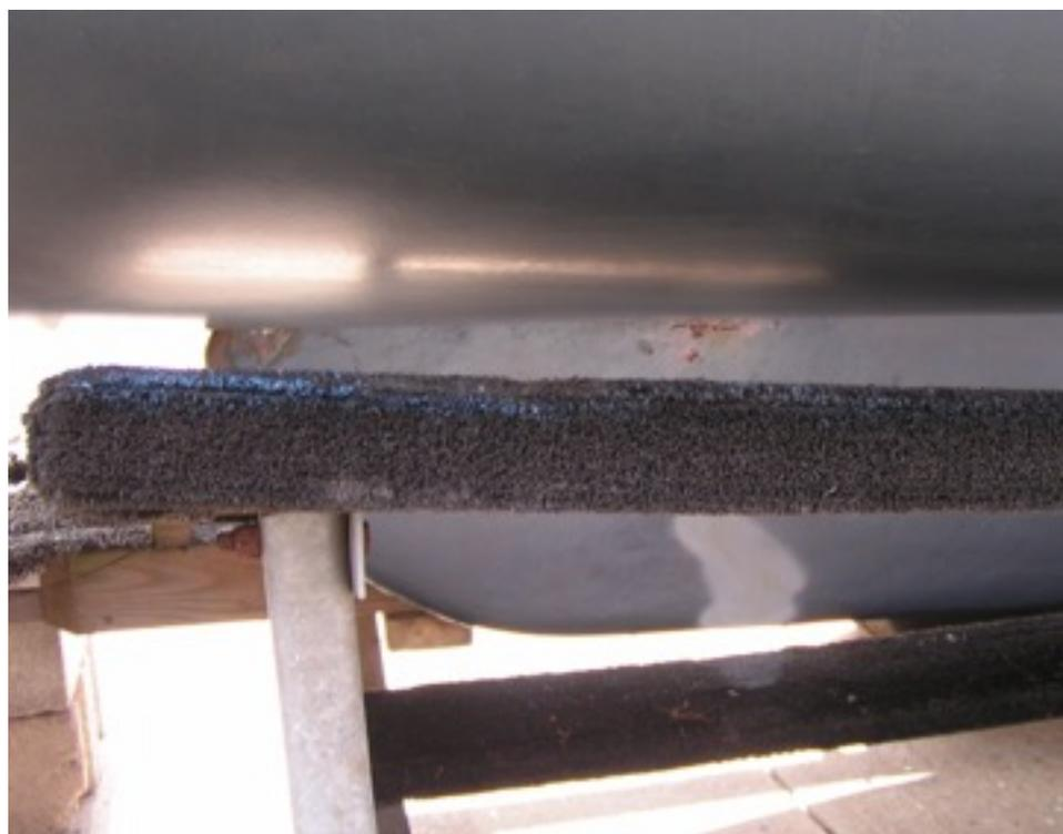
By letting the air out of the trailer tires, this allowed the trailer to set about another 3 inches closer to the ground giving me about 5 inches of clearance between the bunks and the hull for painting. With keel cranked up I had this 5 inches for working on the leading edge of the swing keel and when I lowered the keel onto it's bunk the top 2/3 of the back edge was now exposed.
