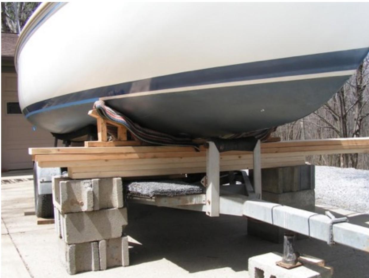
Using just the trailer jack height and supporting the hull, put the hull about 2 inch above the trailer bunks.
