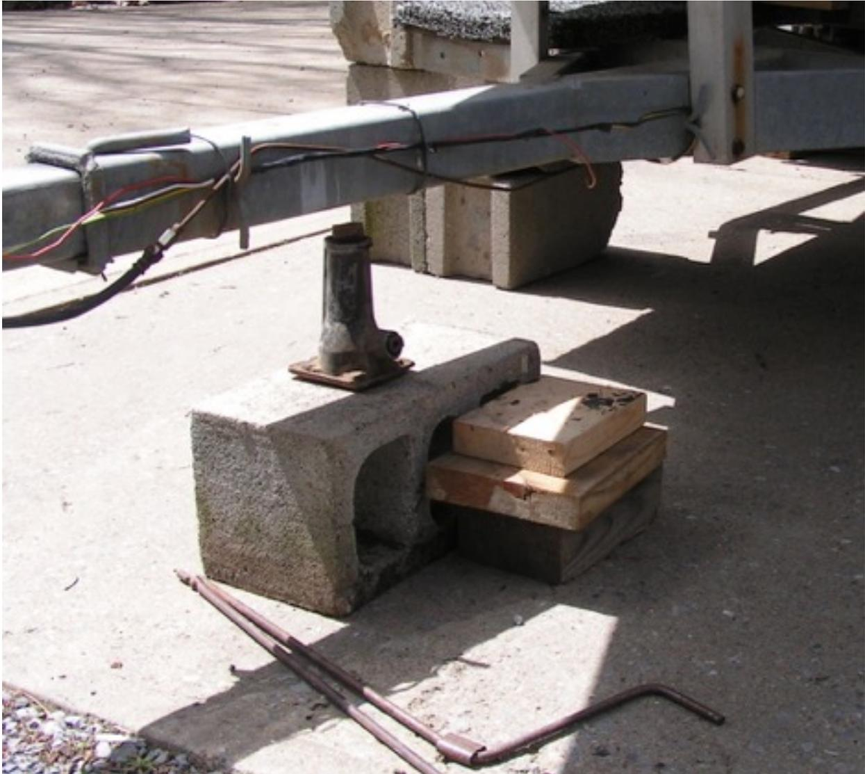
I then used 8 inch concrete blocks to crib up two pillars on each side of the bow just in front of where the trailer narrowed. I then spanned this distance between the pillars with varying lengths of 2x8 and 2x10's. On top of this set a 2x4 V shaped bracket I had made for this boat 21 years ago to hold the bow from rocking sideways when releasing the trailer winch cable and raising the bow above the front ends of the trailer bunks.
