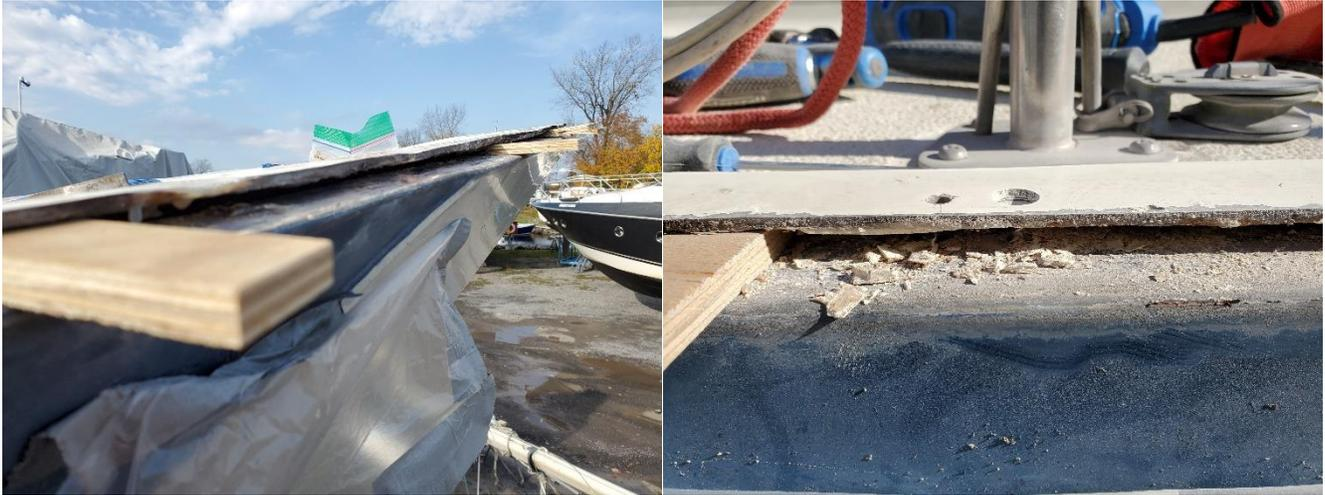
Once it was cleaned out I used 1/8" thick UHMW spacers next to each screw to maintain the gap for the sealant and shot in as much 5200 as I could. I squeezed in a bead at the back of the opening making sure it filled the full height and then squeezed more in to fill the rest of the gap with the nozzle towards the back of the gap using a bit of hydraulic pressure to make sure it filled the entire space.
