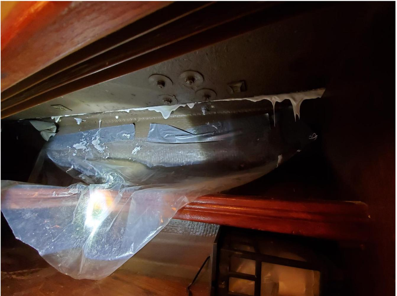
Where the Islander factory used #14 wood screws through the hull to deck joint, I used stainless  $\frac{1}{4}$ -20 x 1.5" countersunk machine screws, flat washers, lock washers and nuts. I haven't decided yet if I will use wood screws or machine screws for the cap rails. Wood screws are much easier but the machine screws weren't bad where they are accessible and are more secure.
