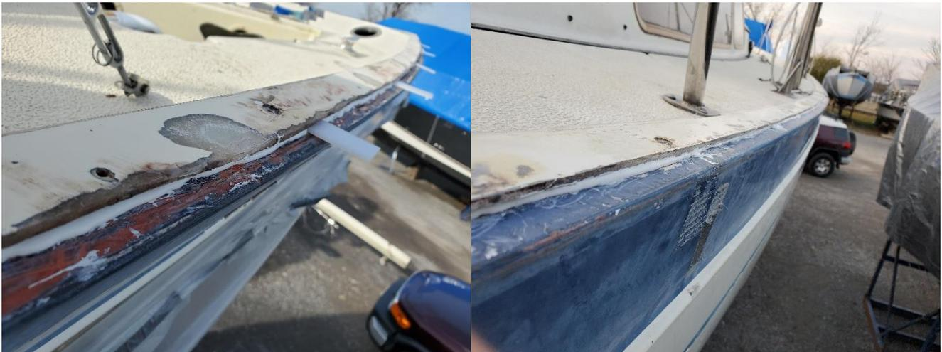
I didn't take pictures of them but there was quite a large gap between hull and deck for the scuppers at the step up between foredeck and aft. I used thickened West Systems G-Flex epoxy to fill this gap. The thickened version is fairly stiff but will still run a bit. I just used tape to hold it in place until it cured. The G-Flex was fairly easy to work with but it's a bit tricky to trowel it in, it's like thick liquid honey. One 8 oz kit was just enough to fill both sides.
