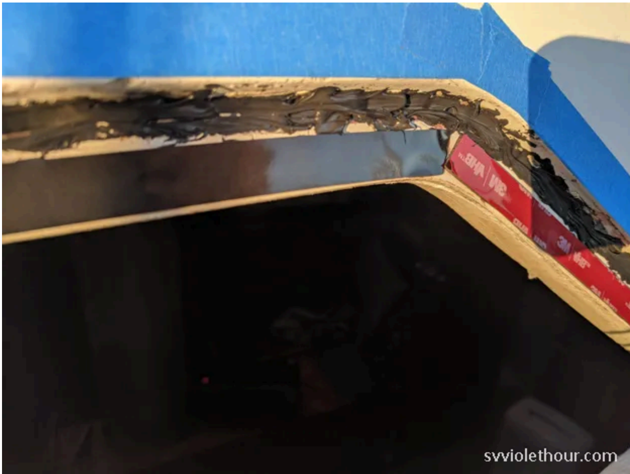
1st window inset, with the 1/2" tape
