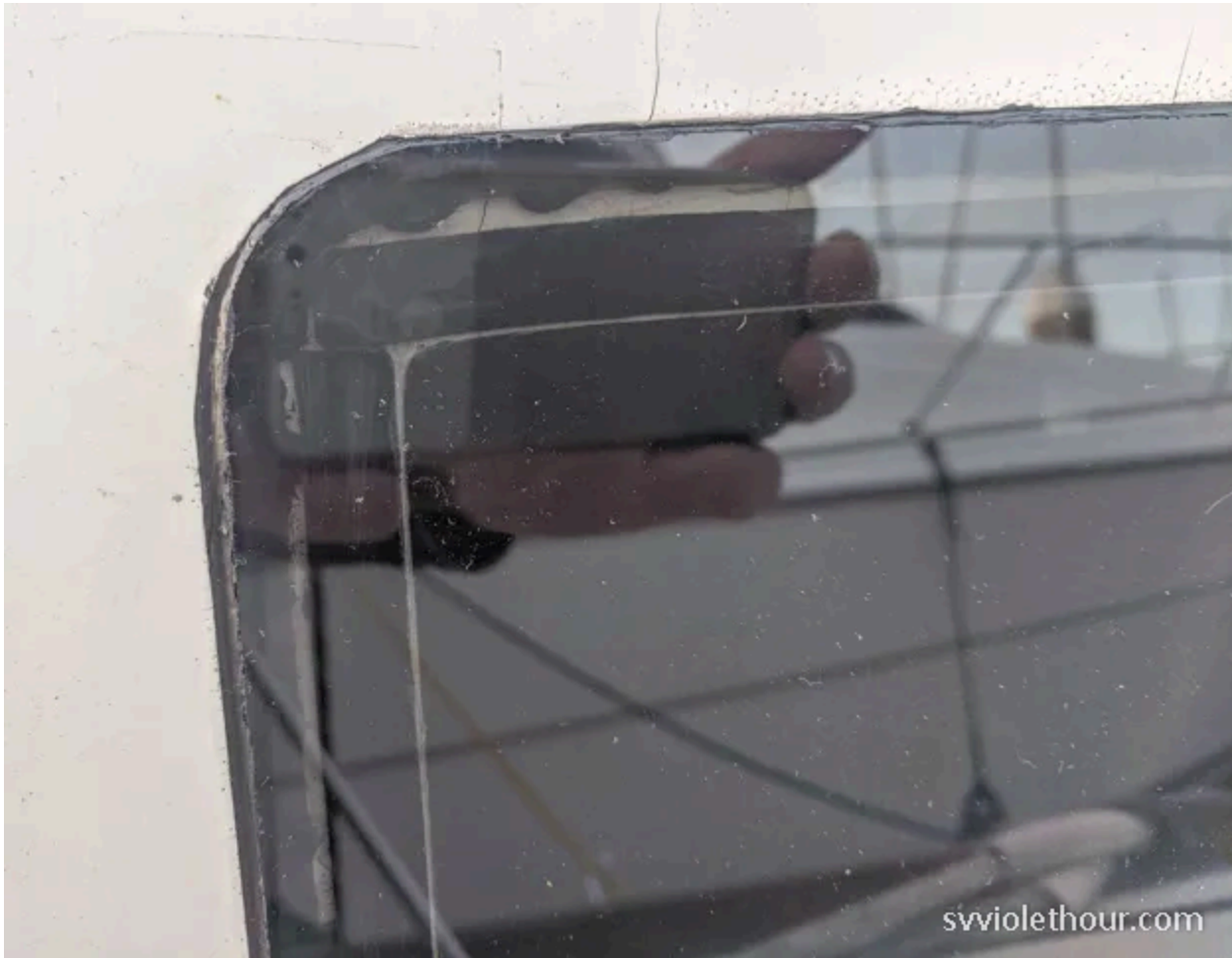
The 1st window, done with 1/2" VHB tape
