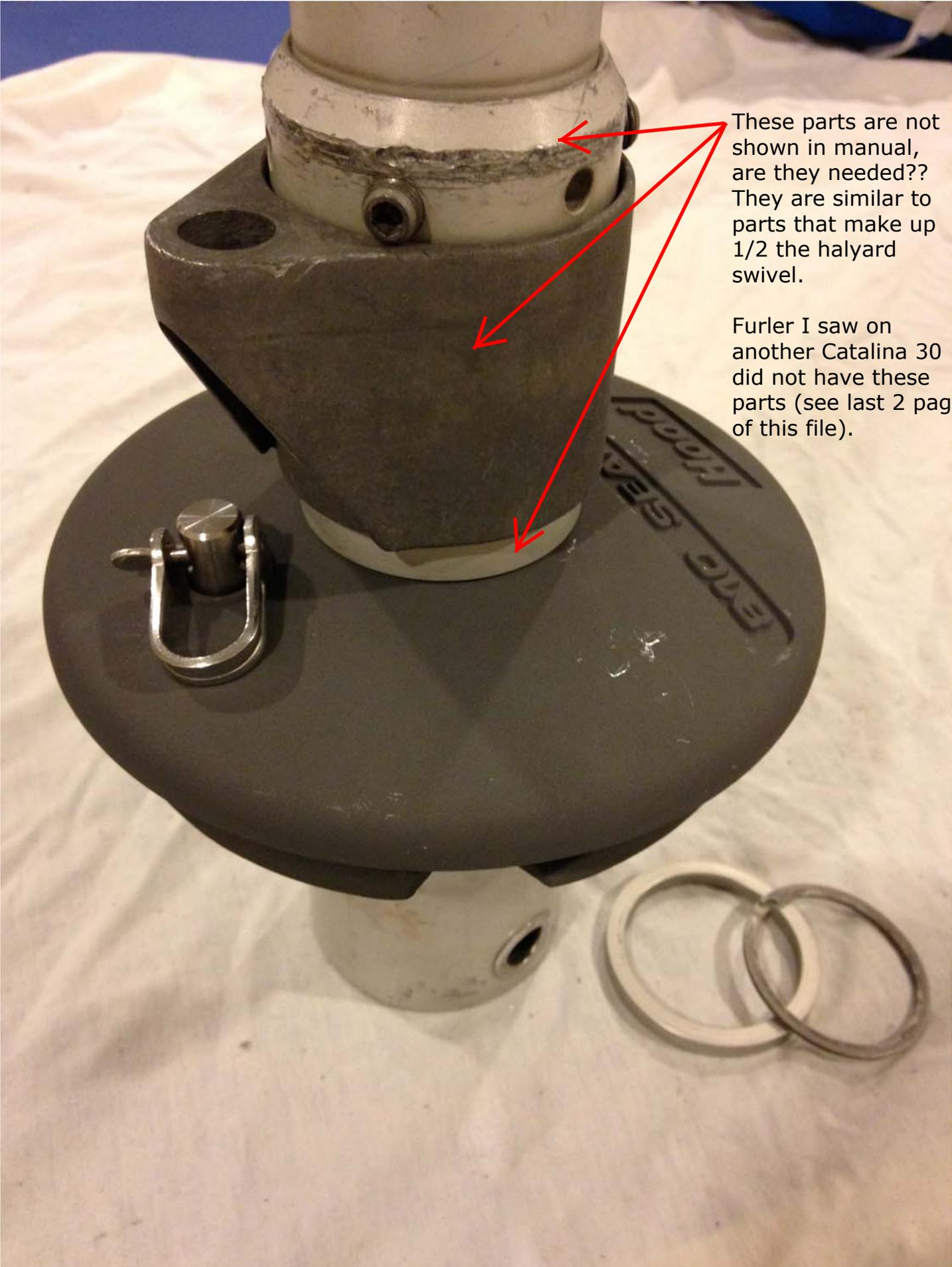
These parts are not shown in manual, are they needed?? They are similar to parts that make up 1/2 the halyard swivel.
