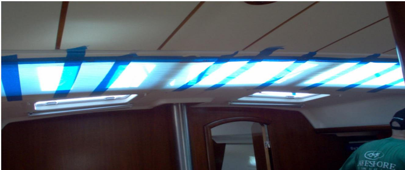
Begin by removing the sealant in one of the corners. Alternating chisel and large screwdriver worked well.
