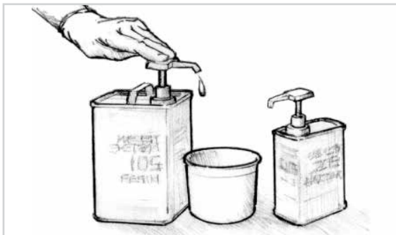
Figure 16-4 Dispense the proper proportions of resin and hardener.
