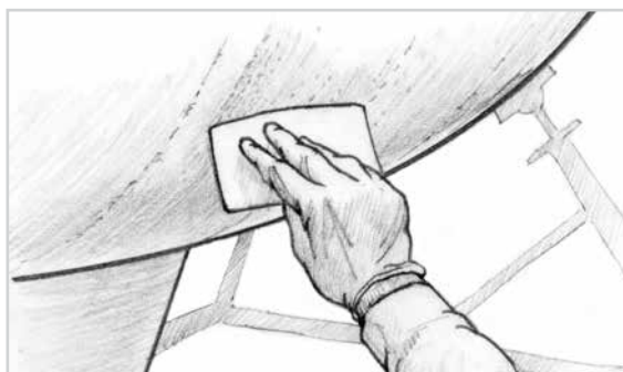
Figure 4 Use a plastic squeegee to press the fabric securely against the hull.
