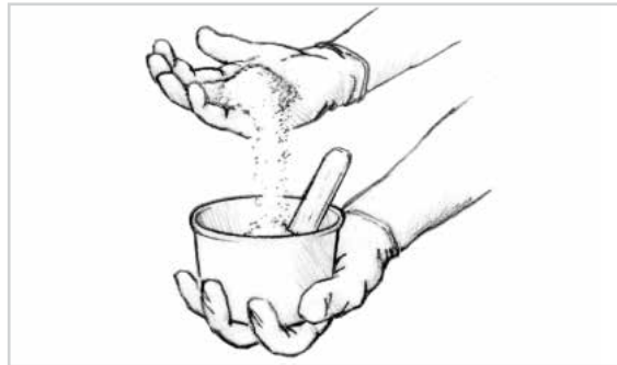
Figure 16-7 Blend in small handfuls or scoops of the appropriate filler until the desired consistency is reached.
