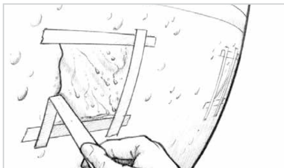
Figure 11-2 A piece of plastic taped to a wet hull will show condensation on the inside of the plastic.
