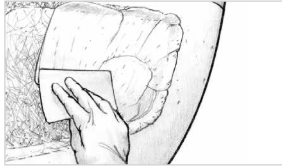
Figure 12-13 Apply a layer of epoxy/406 thickened to a mayonnaise consistency.
