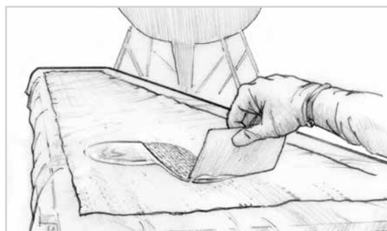
Figure 2 Wet out the fabric by pouring epoxy onto it and spreading it out with a plastic spreader
