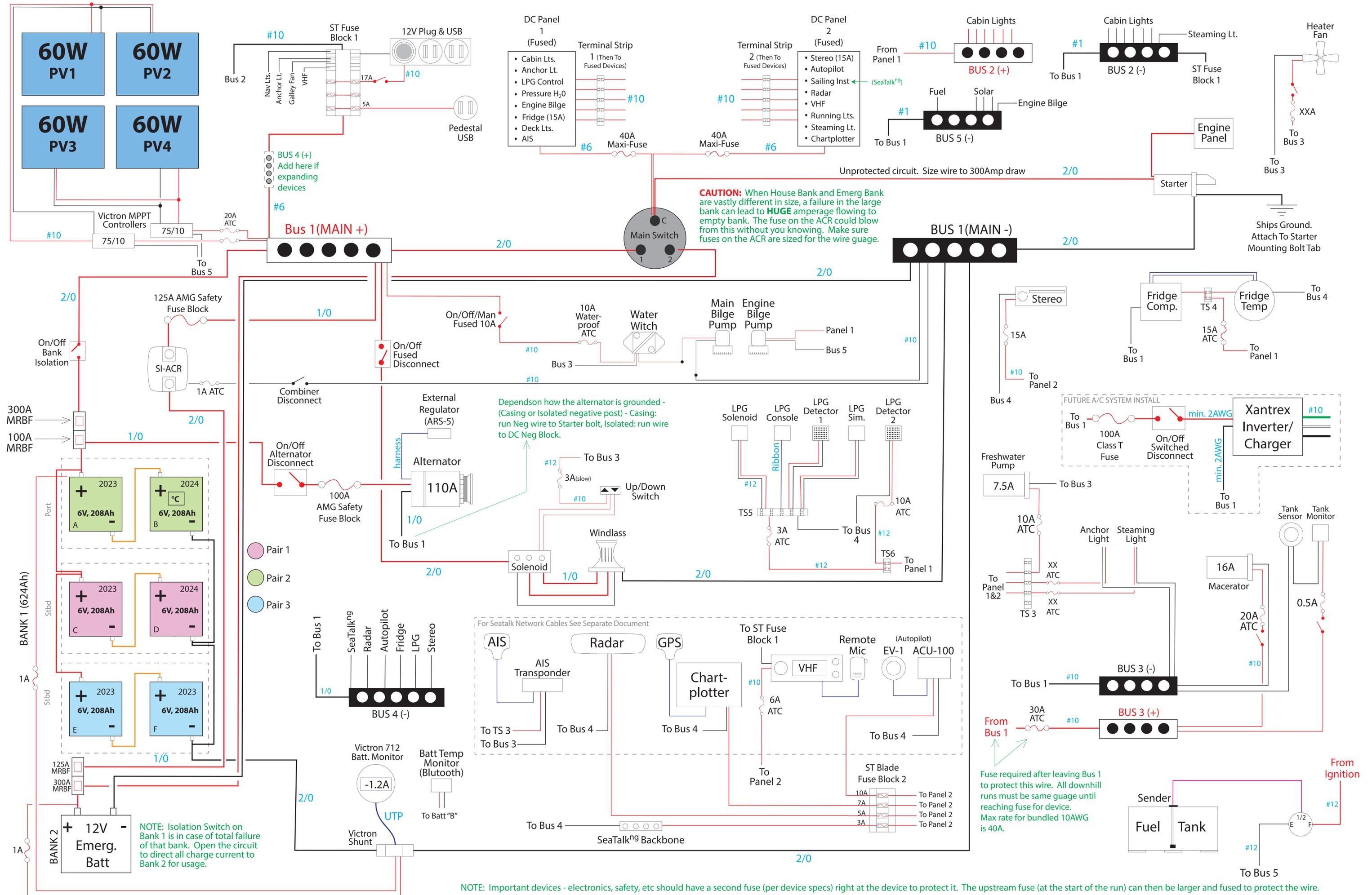
**CAUTION:** When House Bank and Emerg Bank are vastly different in size, a failure in the large bank can lead to **HUGE** amperage flowing to empty bank. The fuse on the ACR could blow from this without you knowing. Make sure fuses on the ACR are sized for the wire guage.
