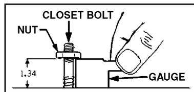
touch top of gauge. If gauge is misplaced, bottom surface of nuts should be 1.34 in. (3.4 cm) above floor.
