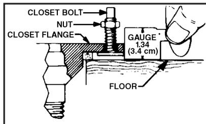
nuts down until they touch top of gauge. If gauge is misplaced, bottom surface of nuts should be 1.34 in. (3.4 cm) above floor.
