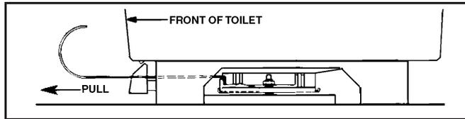
8. If slides cannot be driven by one or two blows, remove toilet and adjust each nut one-half turn upward and repeat procedure from Step 6.
