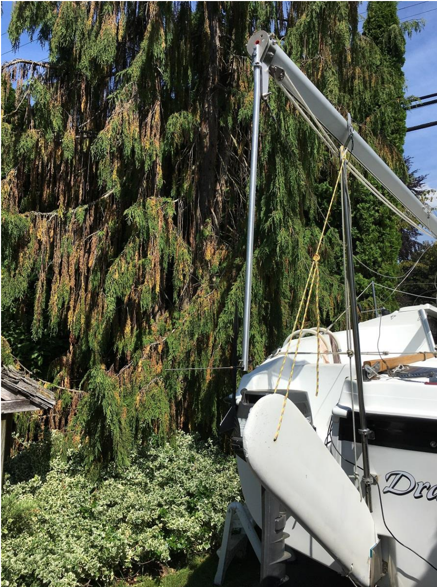
Figure 9: Windex bracket, which positions the Windex within easy reach when the mast is down
