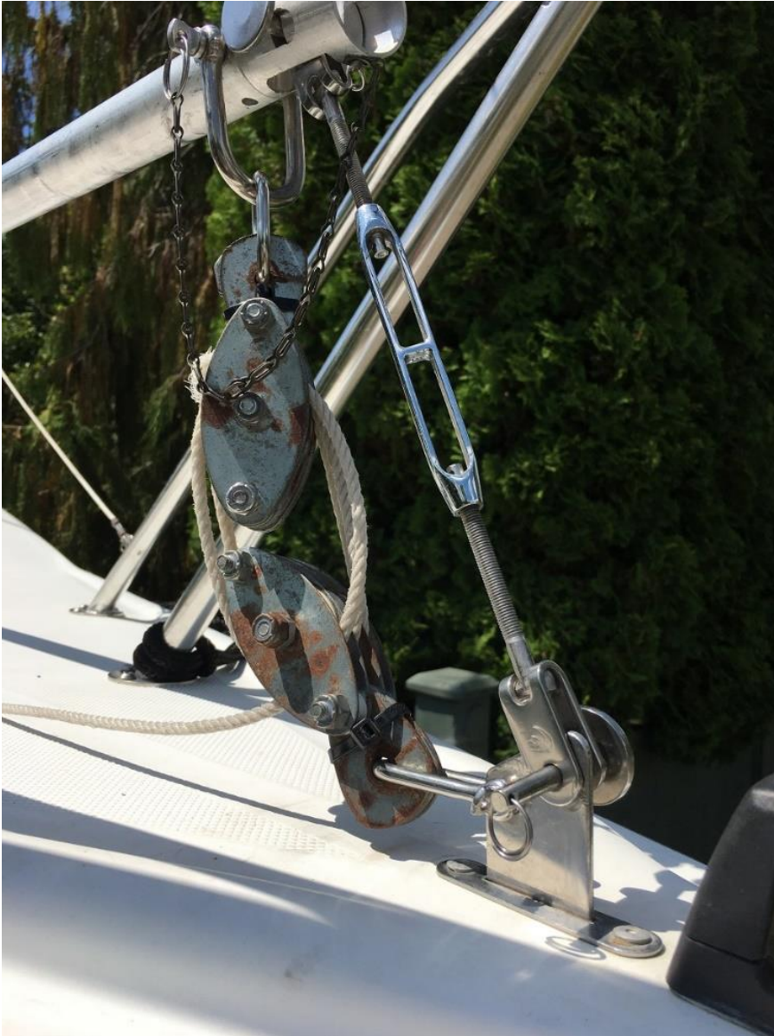
Figure 5: The gin pole positions the forestay turnbuckle so that it can easily be attached to the deck fitting
