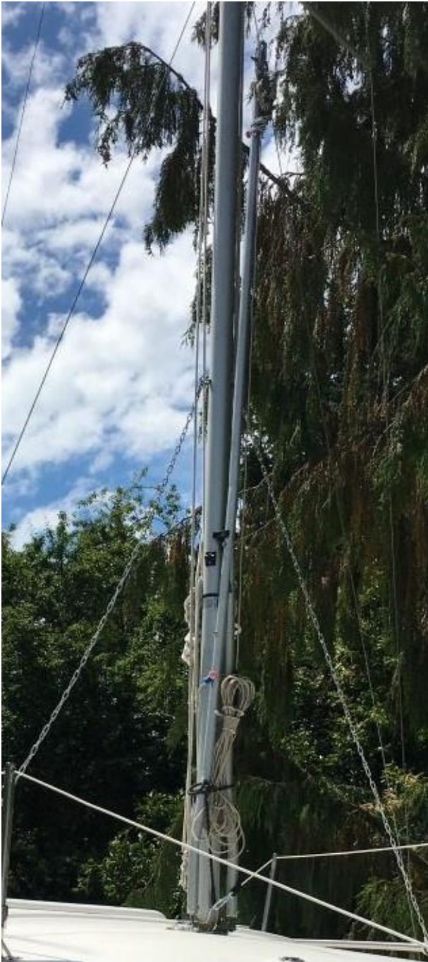
Figure 6: The gin pole secured to the mast, ready for sailing
