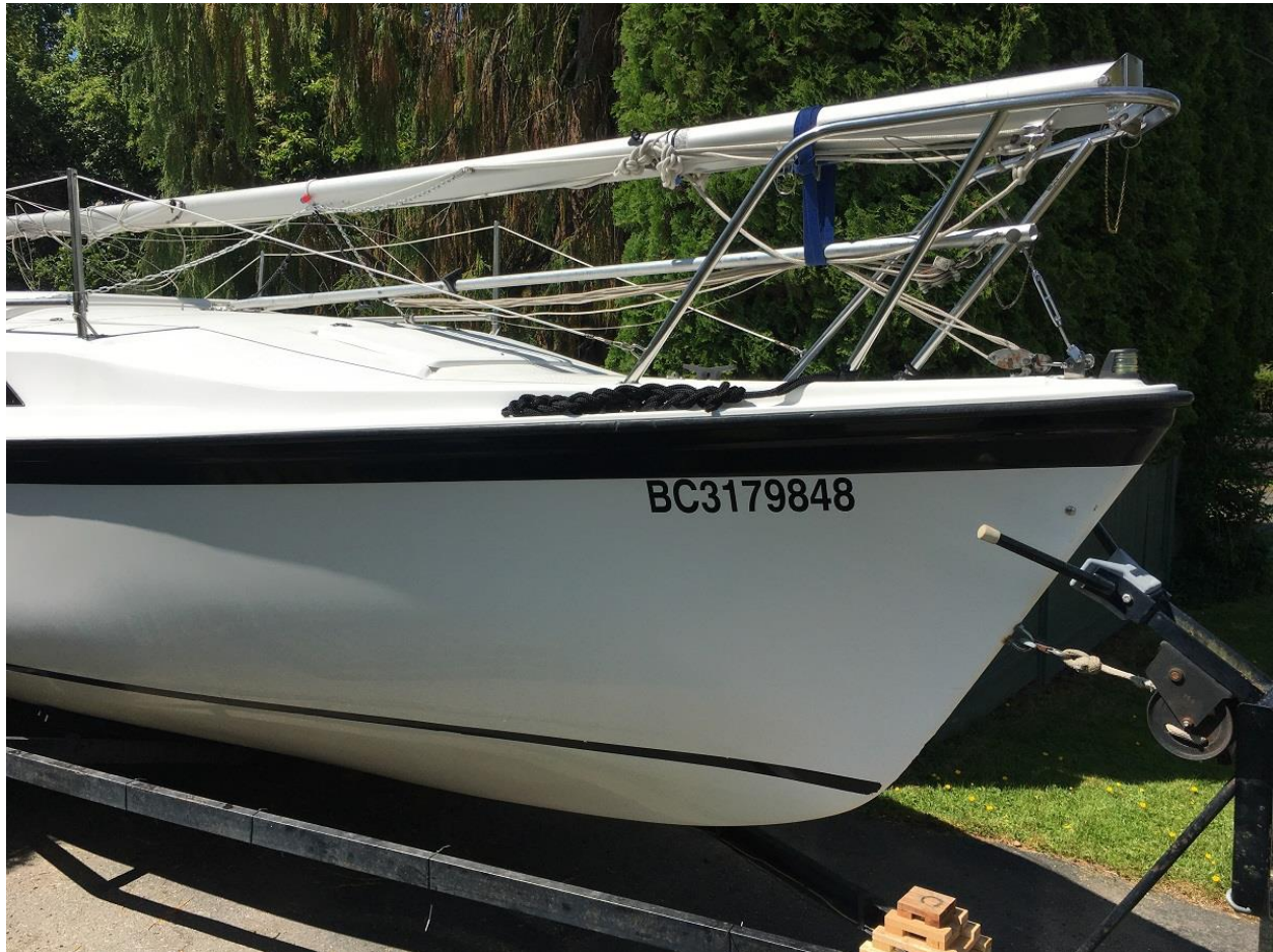
Figure 1: Gin pole, baby stay chains, and B&T as stowed for towing
