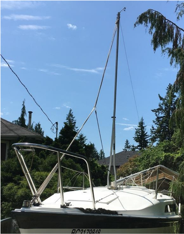
Figure 4: Mast moved back and pinned to foot bracket
