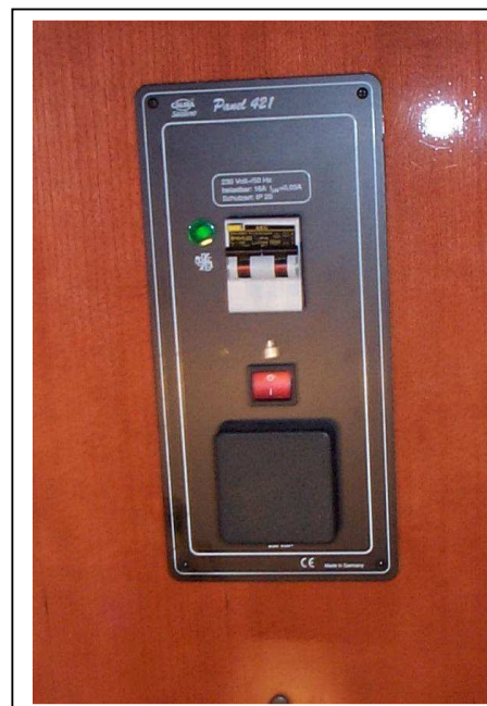
Figure 14: Shore connection panel
