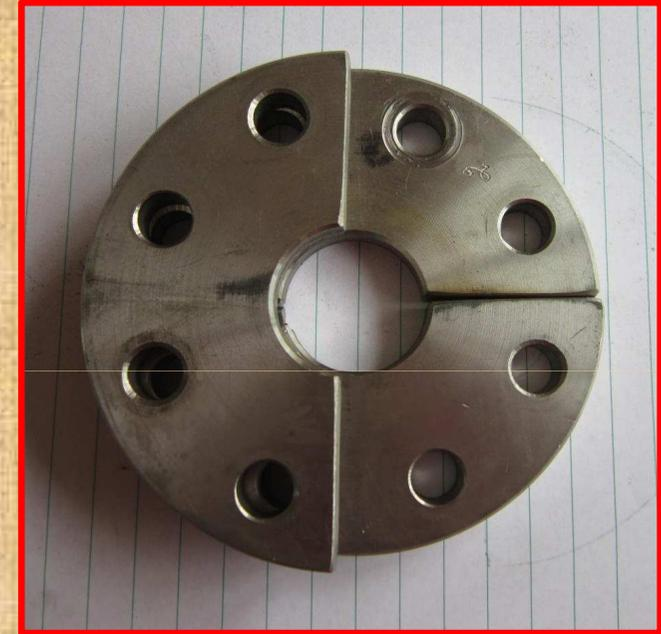
Assemble the 4 plates around shaft, as pictured. Use 4 bolts and tighten being careful that plate is able to slide easily on shaft.
