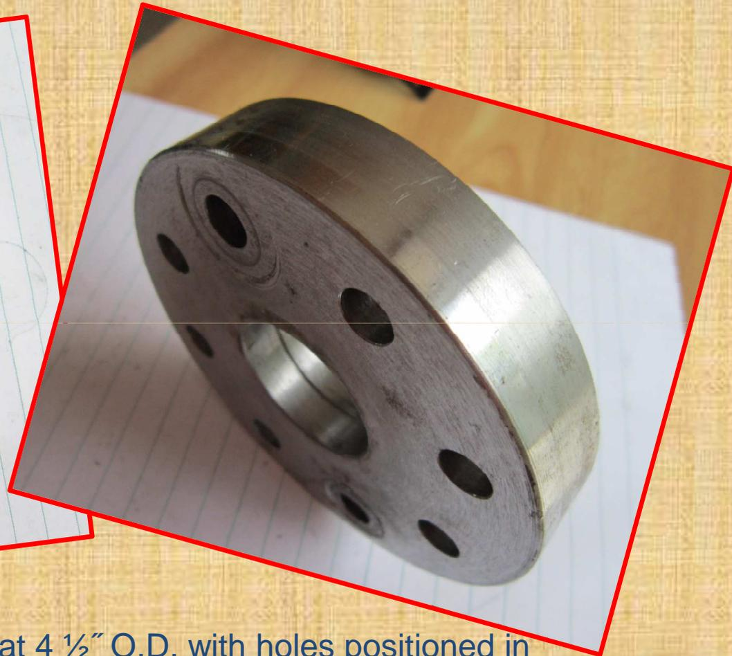
Aft plate is same size at 4 ½" O.D. with holes positioned in same alignment as forward plate. Hole diameter is 1" 5/16
