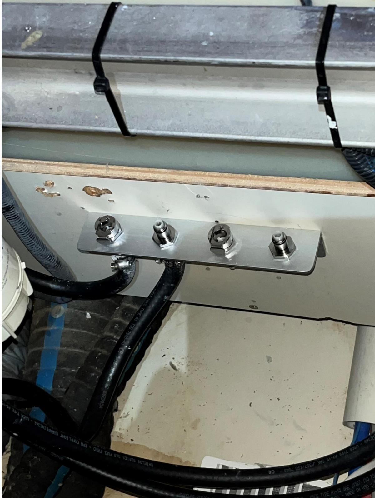
I have chosen the left side (connector) to be “from tank” and the coupling next to it as the “to engine”
