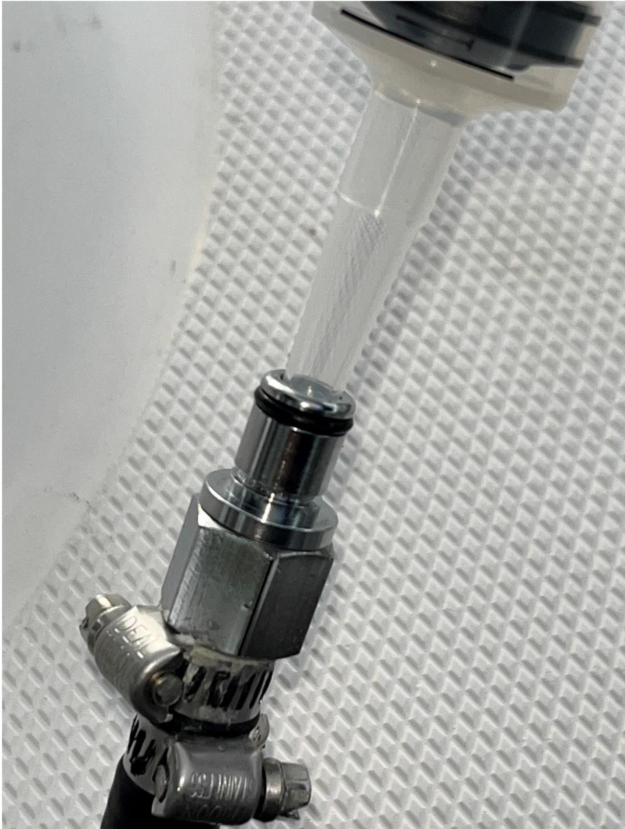
Using the syringe, you will depress the shut off valve, and start to fill the filter with diesel.
