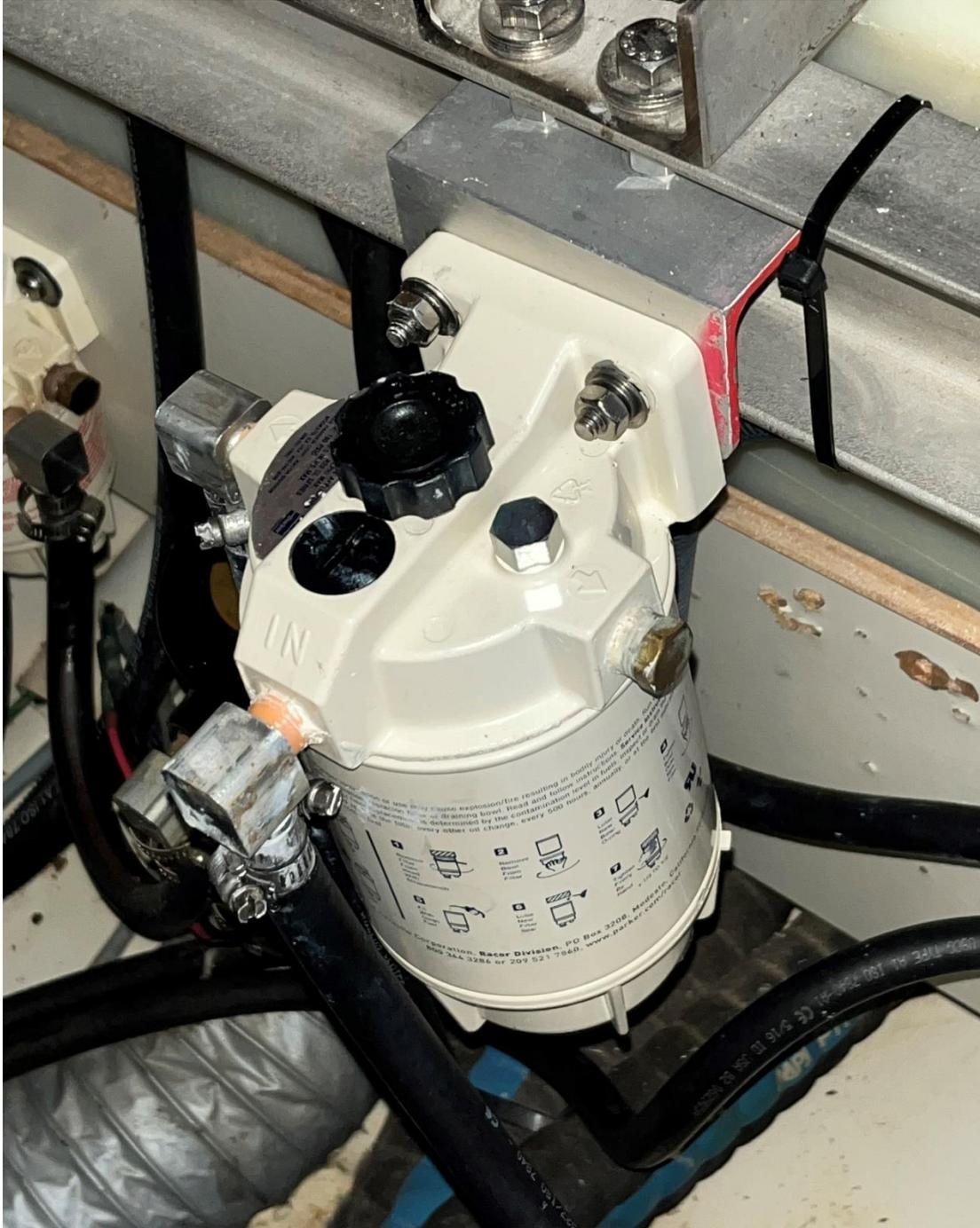
Real simple... I took a short piece of aluminum angle, cut in some ¼-20 threads, wound in some bolts, and now I have a quick on-off mount for the filter. You can do this a thousand different ways. All you want it threaded studs to pop the filter on & off of. You could use a block of wood, starboard, etc. This is super-easy. BTW, you can see the mess of chewed up wood on the panel where the filter used to hang up with short wood screws. Yuk!
