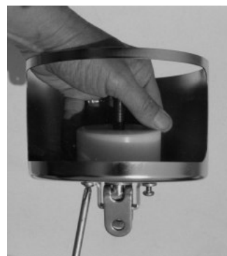
Assembling cup, bearing and antirotation strap
