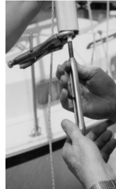
screwing turnbuckle on stud
