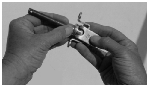
Adding washers to the T-bolt
