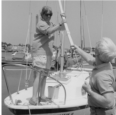
pushing extrusion up forestay
