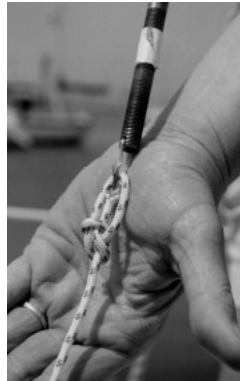
connecting swage stud to messenger line
