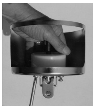
Assembling cup, bearing and antirotation strap
