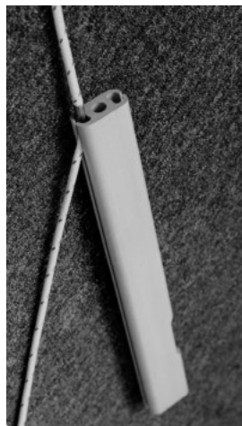
Inserting FF4 ferrule into top of luff
