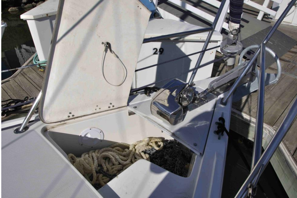
Door Open ( Added wiring access port visible )
