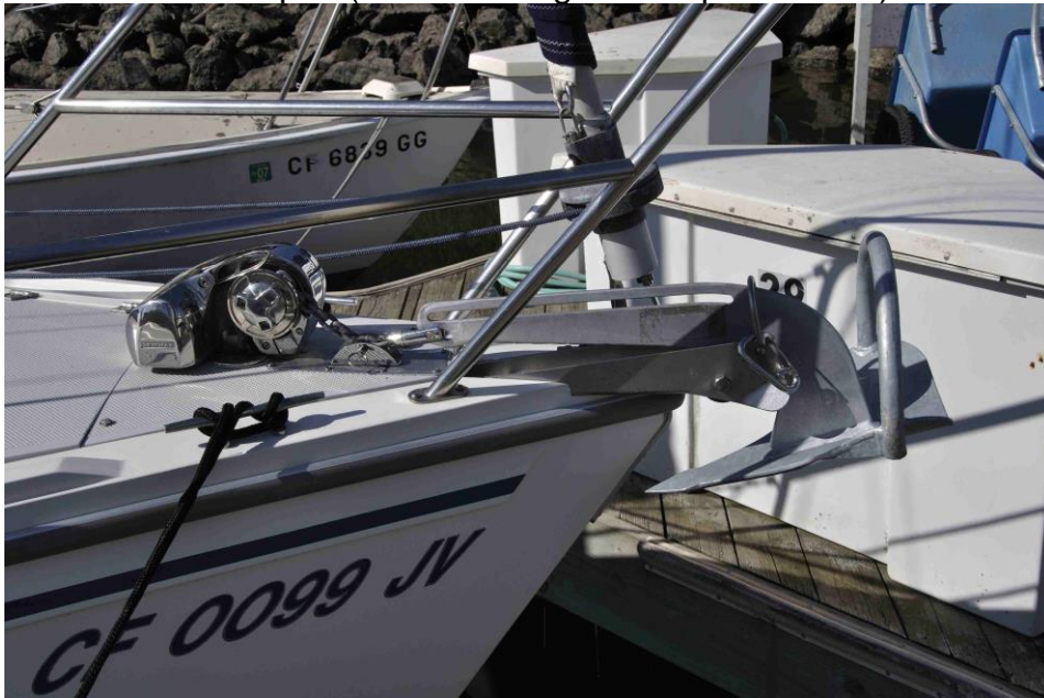
Windlass, new anchor and stopper
