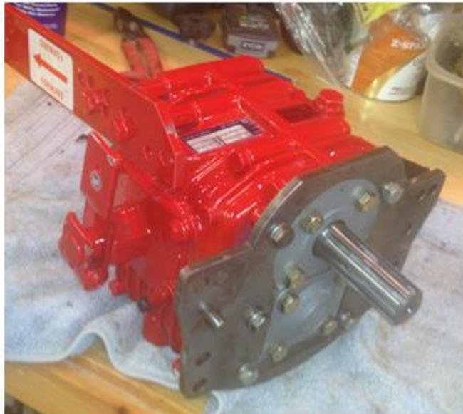
Which is 1" longer than the original. Therefore there is not enough room in the cavity to get the spline shaft straight for insertion.. need about 1" more. Here is the cavity:
