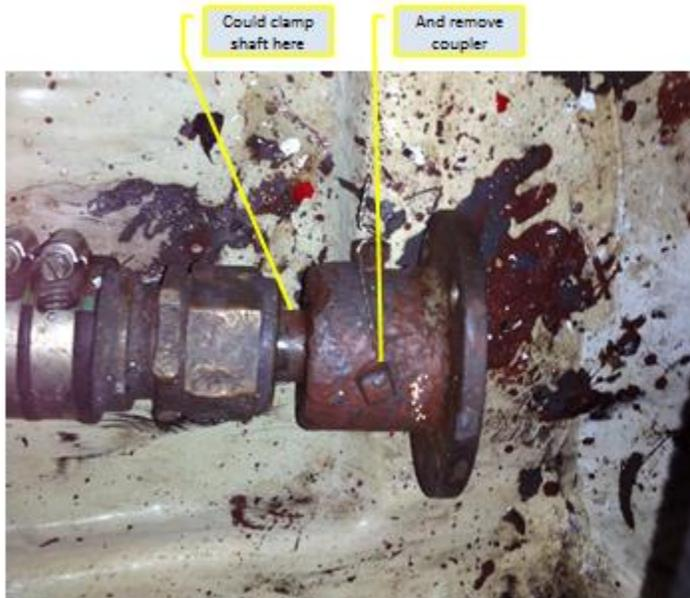
The clamp would prevent the prop shaft from sliding out (and sinking the boat.. it's in the water). There would then be enough room to insert the new xmission. But that seems a little scary and the coupler may not remove that easily... so I'm leaning towards the "c130king" technique.
